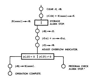
\*As each digit of the partial-word sum is generated, L [i.e., (rC:21)] is counted down. If, at the start, L > s + 1,  $s \neq 0$ , then at the end of the addition (rC:21) will be different from zero, and field overflow will be detected. See Example 6, page 2-27.
