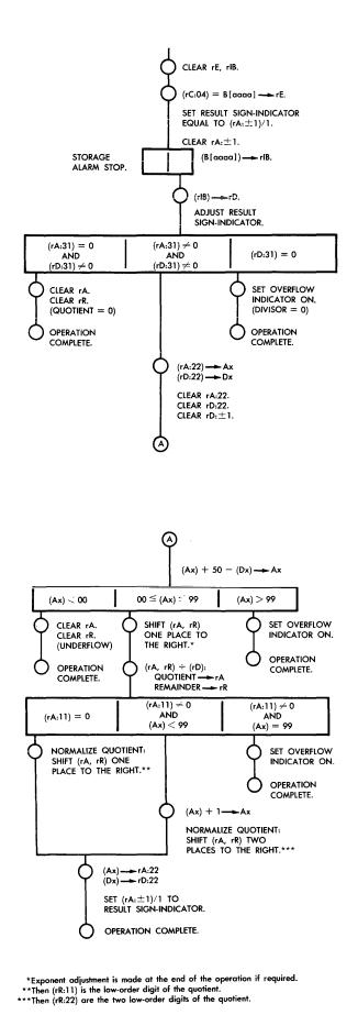
and (B[aaaa]): if the adjusted difference of these exponents is -01, the A and R registers are cleared, and the Execute Phase is terminated, even though normalization of the quotient might yield a valid exponent, namely, 00.
