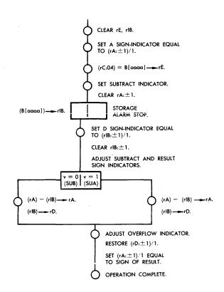
3. If the result of a SUB or SUA instruction is zero, the sign of the result is the same as the one-bit of the sign digit in the A register before execution of the instruction.
