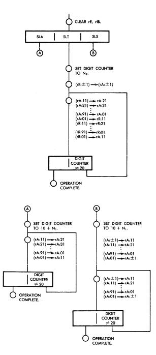
to the left. In this particular case, as will be explained below, the number of digit positions through which the contents of the A register is shifted is eight, of which only seven enter into timing considerations. Examination of the flow chart may help to make clearer the description below.
