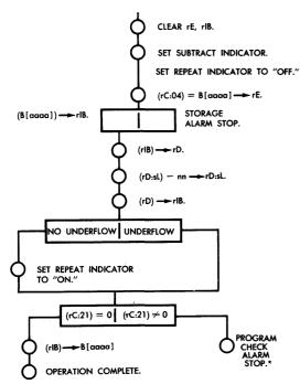
\*As each digit of the partial-word difference is generated, L [i.e., (rC:21)] is counted down. If, at the start, L > s + 1, s ≠ 0, then at the end of the subtraction (rC:21) will be different from zero, and field overflow will be detected. See Example 6, page 2 - 29 -
