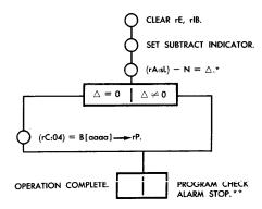
\*The subtrahend, N, is an L-digit number, constructed with the two-digit number, nn, as a basis: the low-order digit of N is the low-order digit of nn; the next-higher-order digit of N is the high-order digit of nn; the next-higherorder digit of N is the low-order digit of nn; and so forth, successively higher-order digits of N being, alternately the high-and low-order digits of nn.
