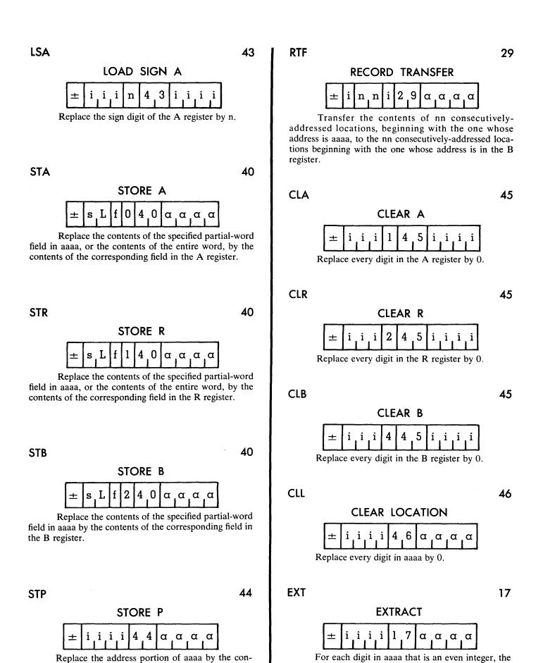
corresponding digit in the A register is replaced by zero.
