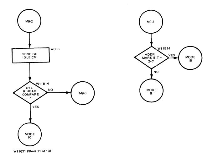
Figure 3-5. Read and Write and Verify Operation (Sheet 11 of 13)
