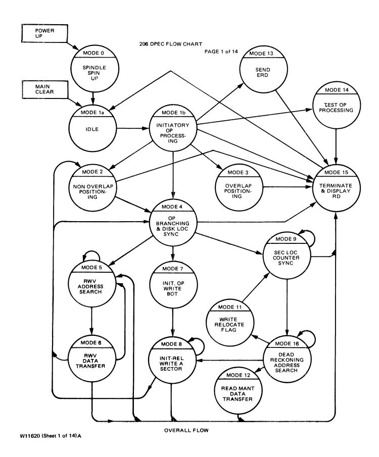
Figure 3-4. Detailed DPEC Flow Chart (Sheet 1 of 14)
