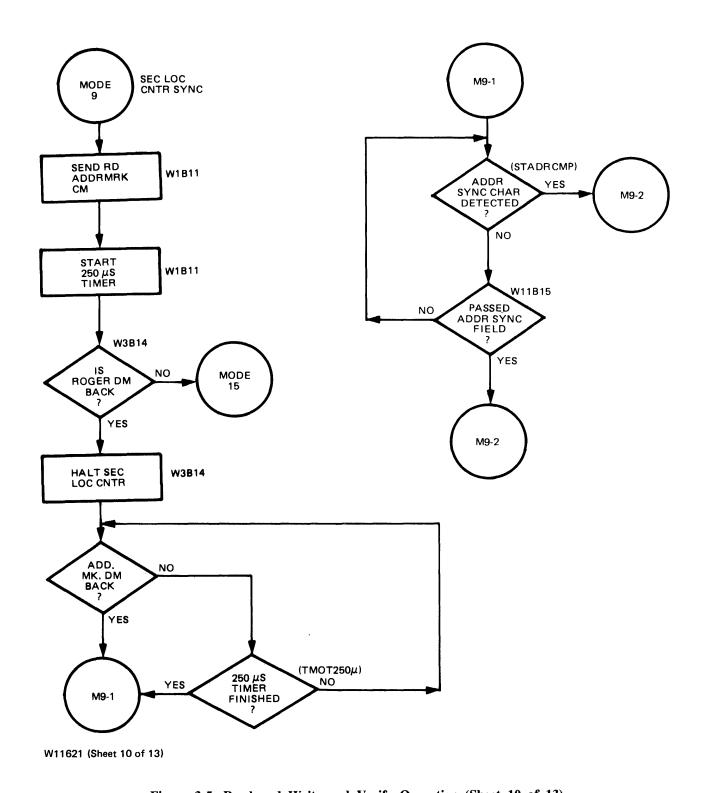
Figure 3-5. Read and Write and Verify Operation (Sheet 10 of 13)
