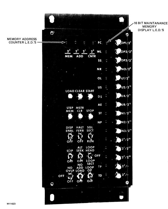
Figure 4-1. Maintenance Control Panel
