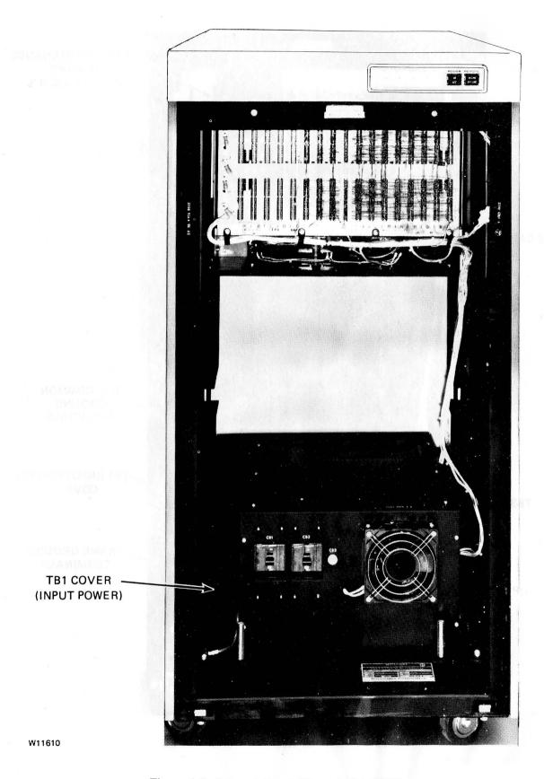
Figure 1-2. Internal Front View of 206 DPEC
