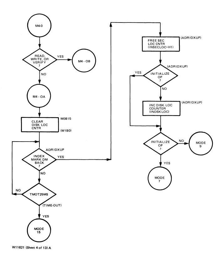
Figure 3-5. Read and Write and Verify Operation (Sheet 4 of 13)
