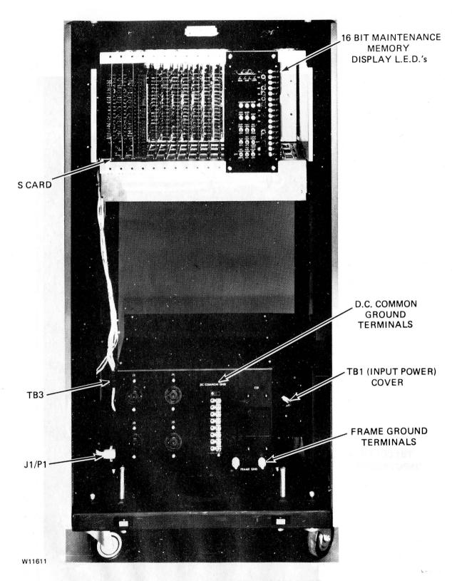
Figure 1-3. Internal Rear View of 206 DPEC
