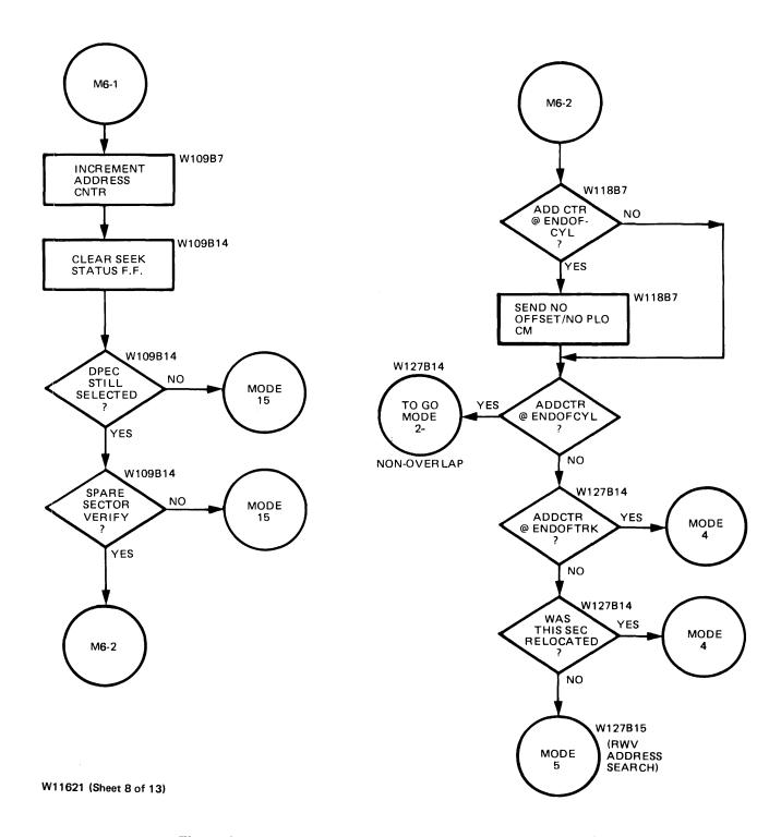
Figure 3-5. Read and Write and Verify Operation (Sheet 8 of 13)
