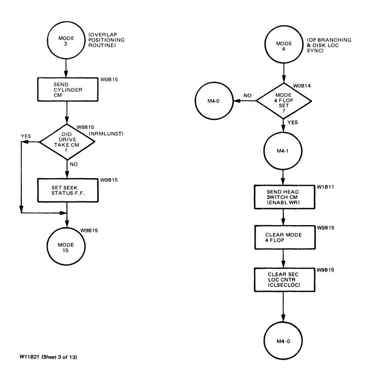
Figure 3-5. Read and Write and Verify Operation (Sheet 3 of 13)
