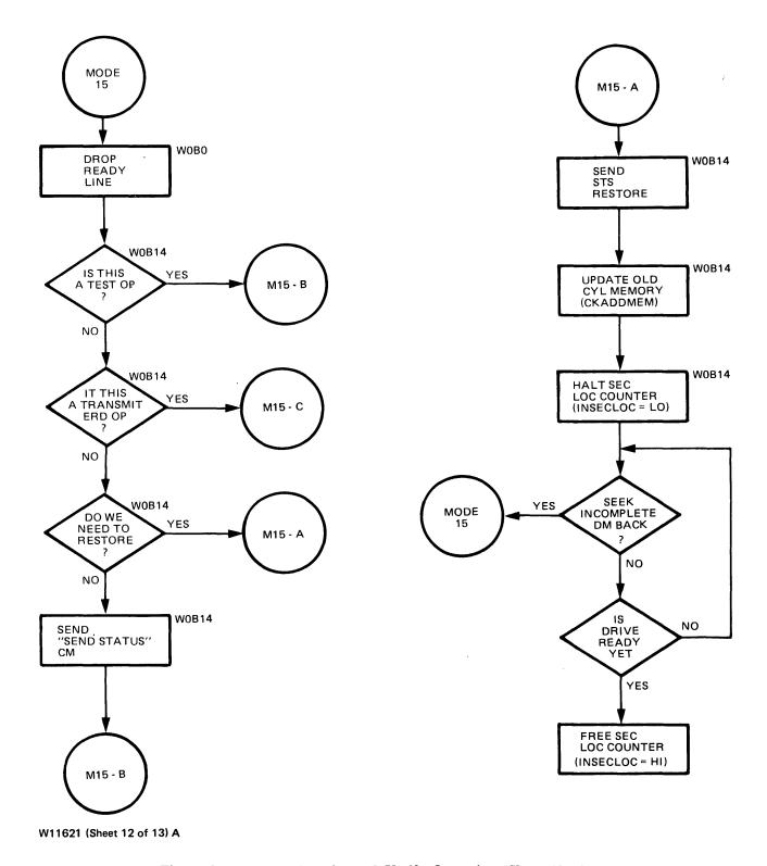
Figure 3-5. Read and Write and Verify Operation (Sheet 12 of 13)
