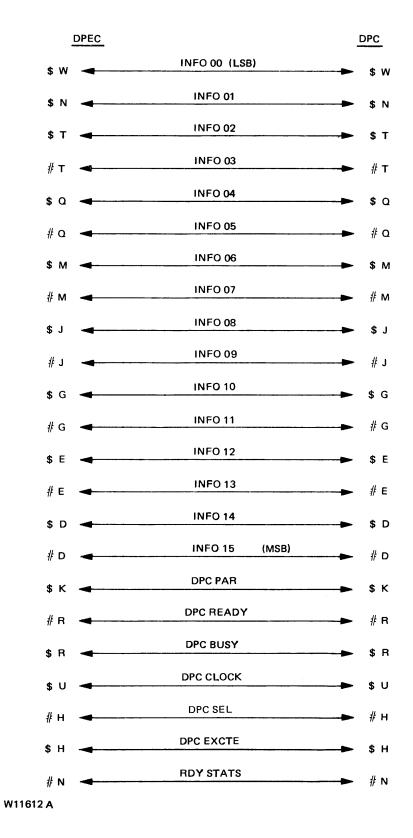
Figure 1-4. Interface Lines, DPEC to DPC ground.
