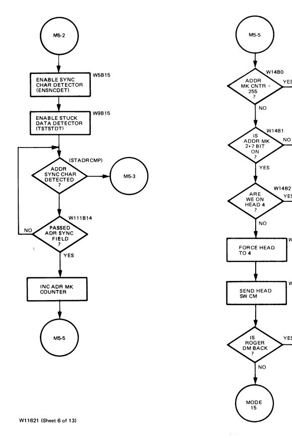
Figure 3-5. Read and Write and Verify Operation (Sheet 6 of 13)
