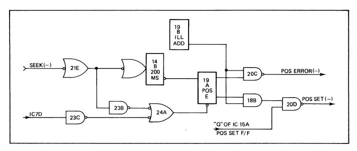
Figure 2-16. Position Error Detection.
