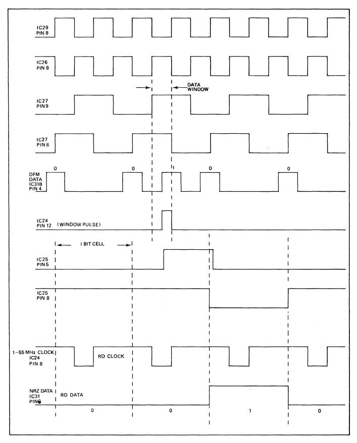
Figure 2-27. Data Discriminator. Window (Strobing) Timing And Decoding
