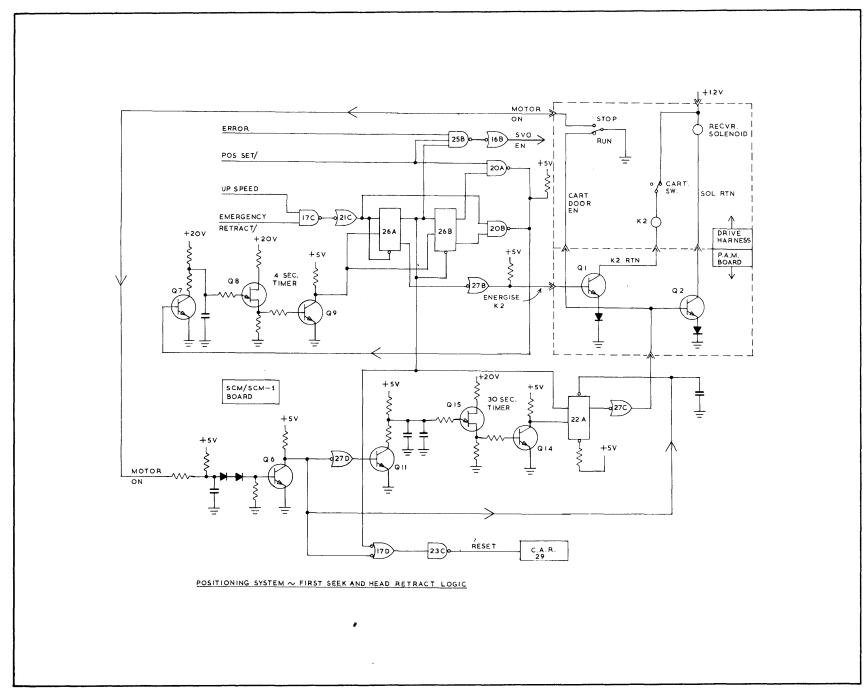
Figure 2-2. Positioning System First Seek And Head Retract Logic
