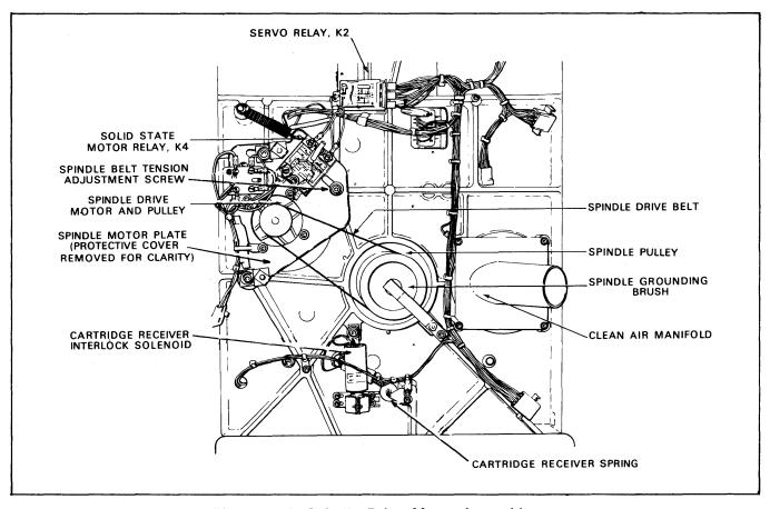
Figure 5-19. Spindle Drive Motor Assembly
