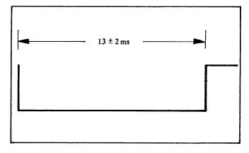
Figure 4-6. Short Servo Gate
