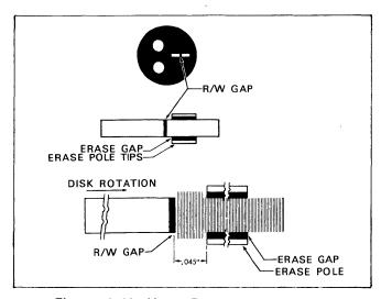
Figure 1-13. Head Recording Principles
