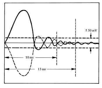
Figure 4-9. Servo Settle Time
