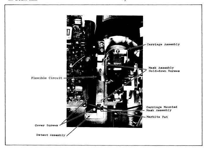
Figure 5-10. Detent Assembly
