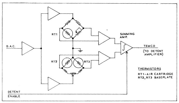
Figure 1-23. Temperature Compensation Network - Block Diagram
