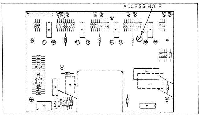
Figure 4-20. Location of Access Hole for R133 (SCM-2 board)
