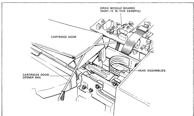
Figure 1-7. Disk Cartridge in Place in Drive Module
