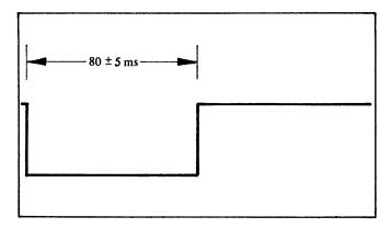
Figure 4-8. Long Servo Gate - Width
