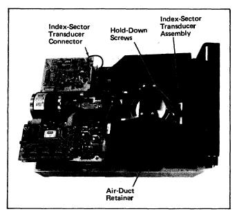
Figure 5-17. Index/Sector Transducer Assembly
