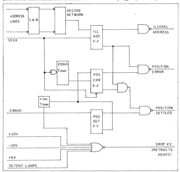
Figure 1-21. Positioning System - Control and Error Detection Logic Block Diagram
