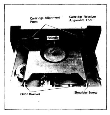
Figure 5-18. Receiver Alignment Tool
