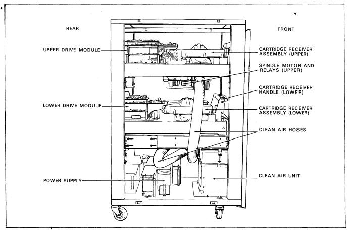
Figure 1-2. Side View of Drive Cabinet (Panel Removed)
