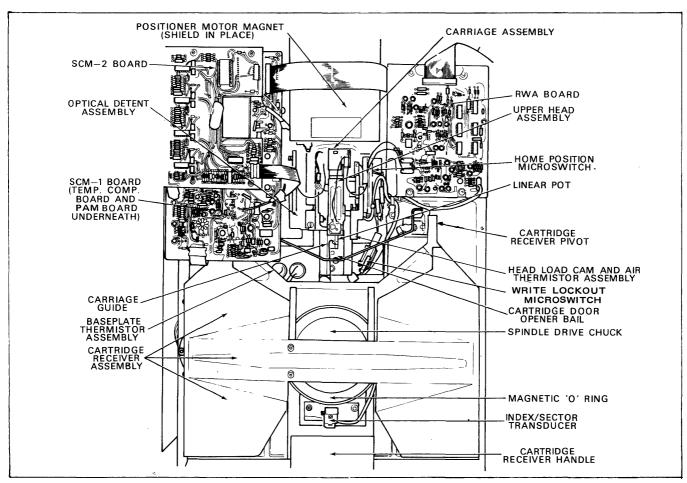
Figure 1-10. Plan View of 9481-12 Drive Module
