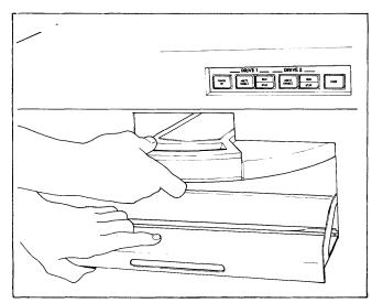
Figure 1-6. Inserting a Disk Cartridge into the Receiver (Upper Drive Module)
