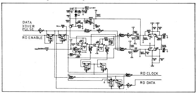
Figure 2-22. Data Discriminator and Phase Locked Loop (Part of CEM Board)
