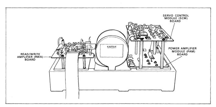
Figure 1-24. Rear View of Module Showing Boards (9480-12)
