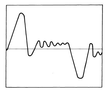
Figure 4-10a. Servo Offset Adjustment - Incorrect
