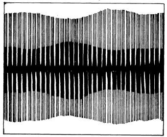
Figure 4-11a. Dibit Pattern-Head Alignment-Incorrect
