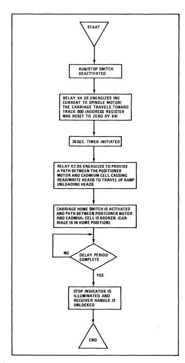
Figure 2-6. Power-Down And Head Retraction Flow Chart
