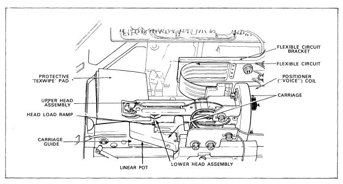
Figure 1-18. Positioner Mechanism (with protective pad in place between heads)
