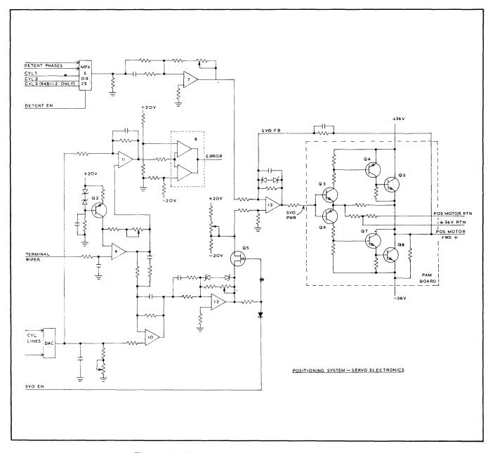
Figure 2-8. Positioning System Servo Electronics
