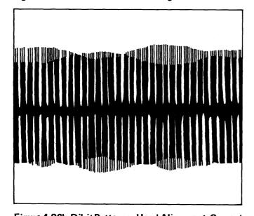
Figure 4-26b.Dibit Patterns - Head Alignment-Correct
