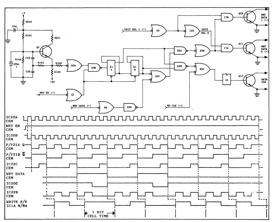
Figure 2-18. Write Data Encoder Part of CEM
