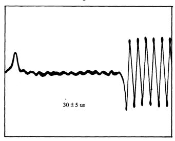
Figure 4-27.INDEX-to-Data Burst (Radial Alignment)
