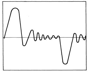
Figure 4-25b. Servo Offset Adjustment - Correct
