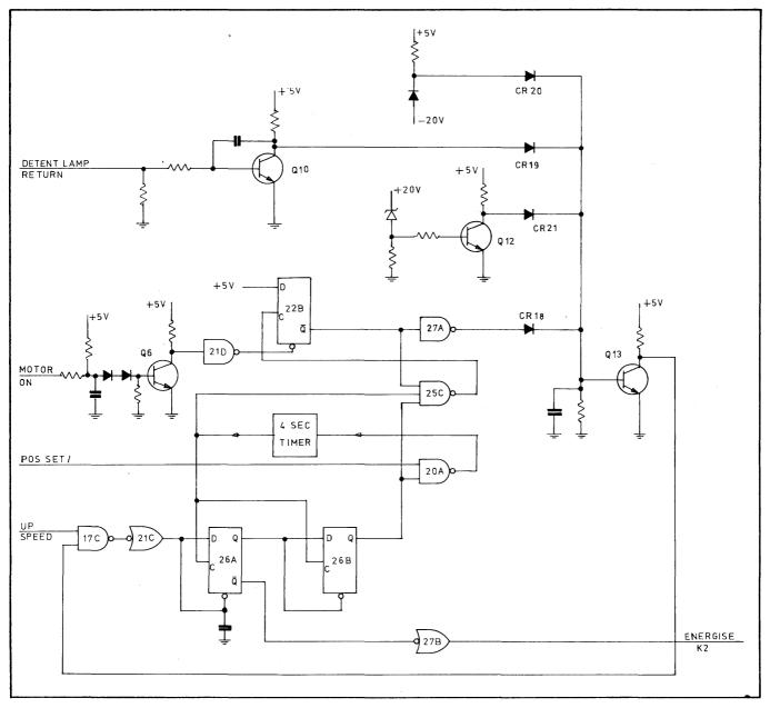
Figure 2-15. Failure Detection Circuitry.
