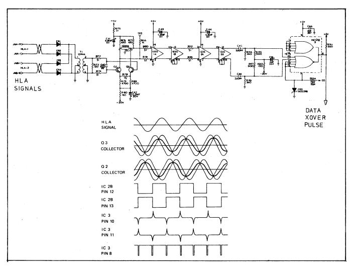
Figure 2-21. Head Signal Discriminator (Part of CEM Board)
