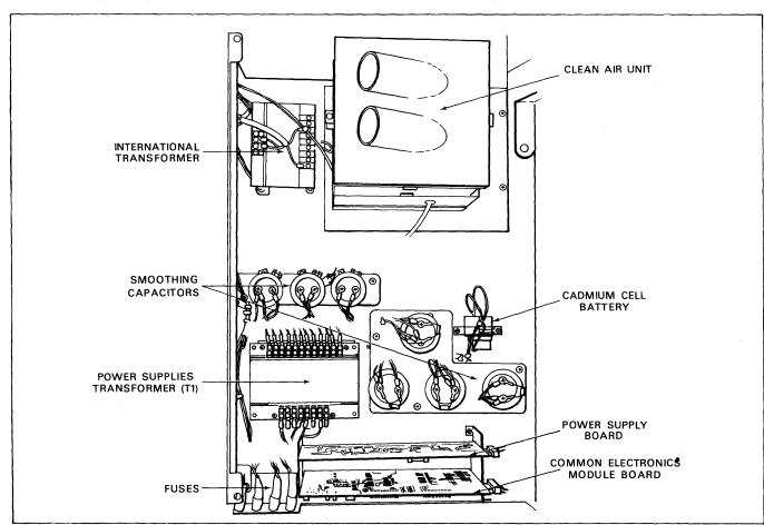
Figure 1-3. Plan View of Power Supply Area
