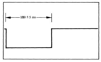
Figure 4-23. Long Servo Gate - Width
