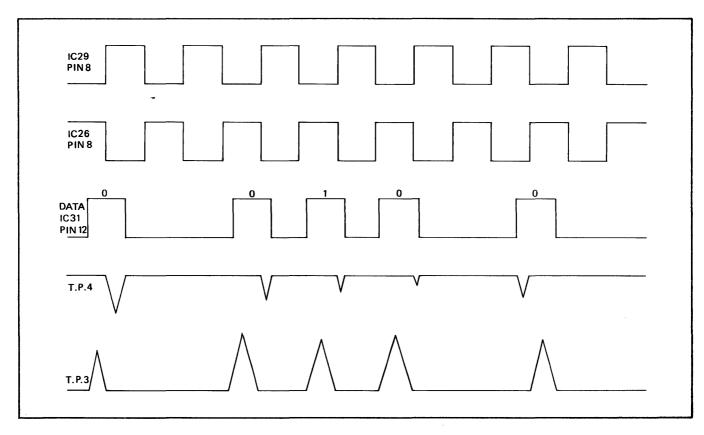
Figure 2-25. Phase-Locked Loop Timing Chart Data Frequency Too High (Disk Rotating Faster)
