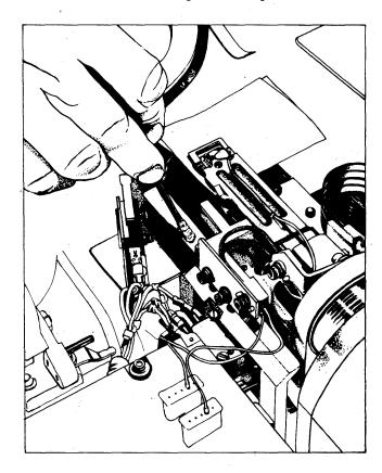
Figure 4-4. Cleaning Carriage Guide and Linear Pot
