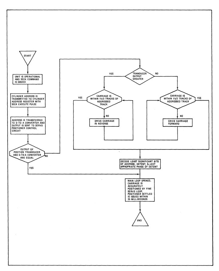
Figure 2-7. Operational Flow Chart Programmed Seek
