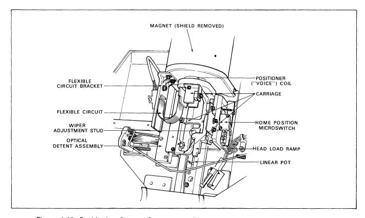
Figure 1-19. Positioning System Components (Heads and Boards Removed for Clarity)
