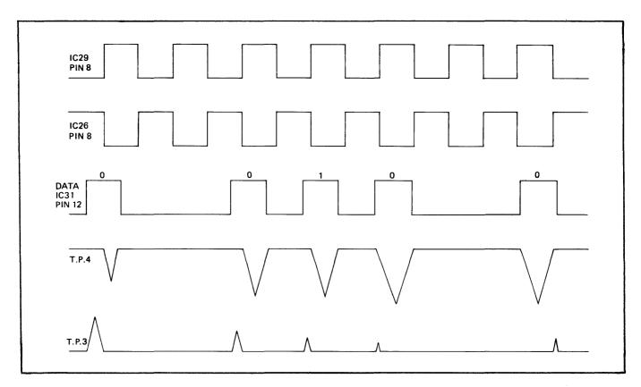
Figure 2-24. Phase-Locked Loop Timing Chart Data Frequency Too Low (Disk Rotating Slower)
