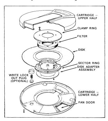
Figure 1-5. Disk Cartridge (Exploded View)
