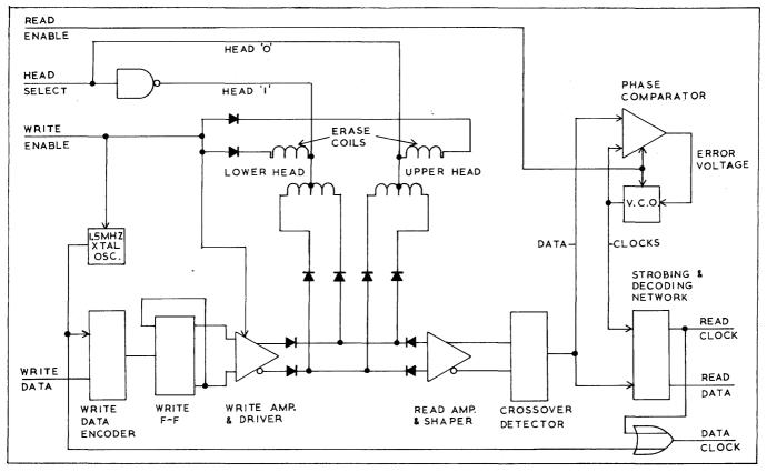
Figure 1-22. Read-Write System - Simplified Functional Block Diagram
