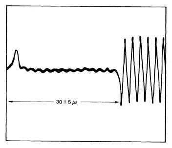
Figure 4-12. INDEX-To-Data Burst (Radial Alignment)
