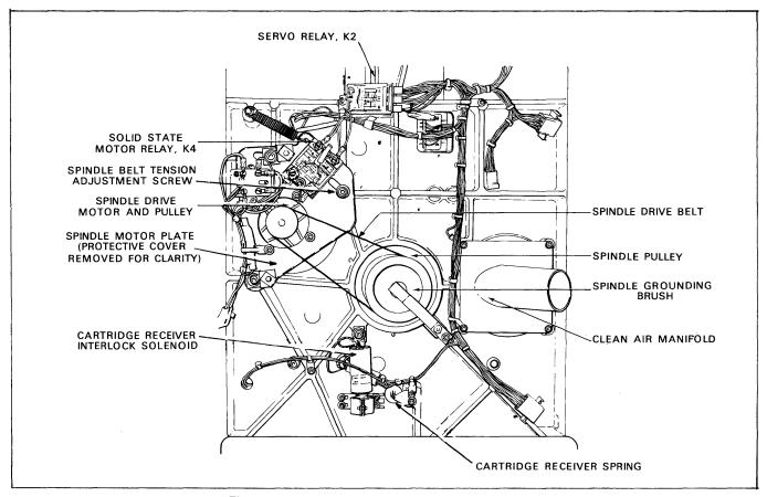
Figure 1-11. Bottom View of Drive Module
