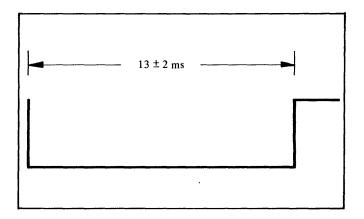
Figure 4-21. Short Servo Gate.
