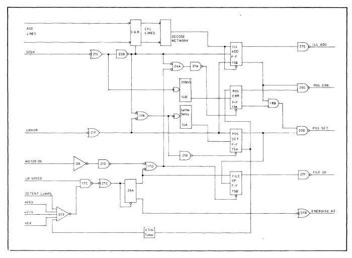
Figure 2-9. Positioning System. Control And Error Detection Logic.
