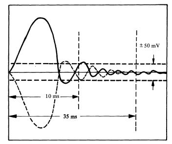
Figure 4-24. Servo Settle Time
