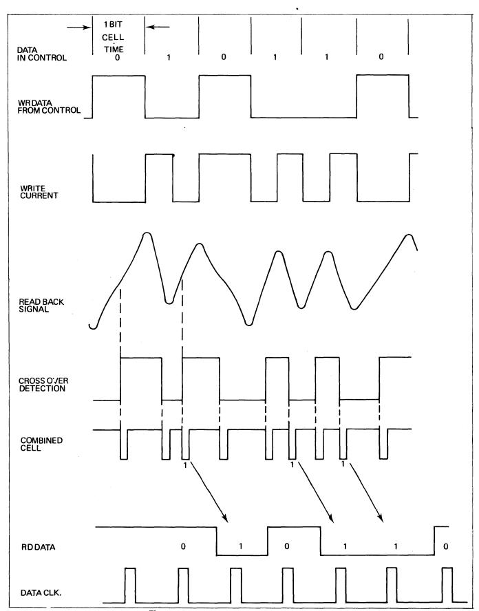
Figure 1-14. Double Frequency Recording
