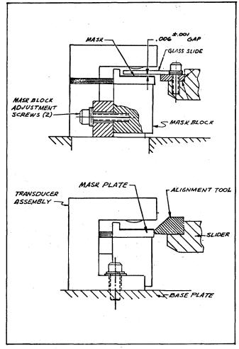
Figure 5-15. Positioning of Detent and Mask Assemblies (9481-12 Only)
