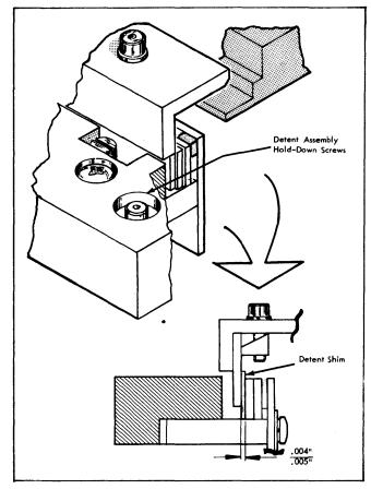
Figure 5-13. Positioning of Detent and Mask Assemblies (9480-12)
