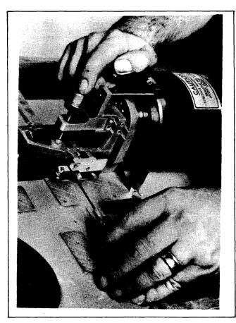
Figure 5-12. Transducer Wiper Adjustment Tool
