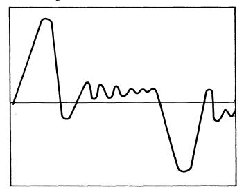
Figure 4-25a. Servo Offset Adjustment - Incorrect
