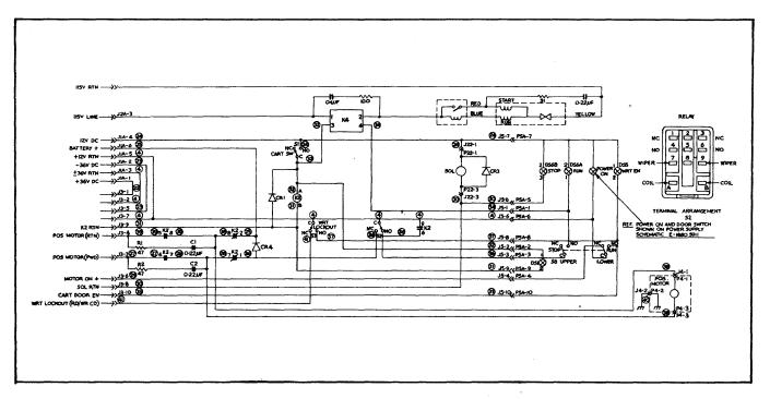
Figure 2-3. Main Harnesses, Switches And Relays.
