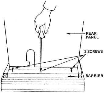
Figure 6-2. Removing Barrier
