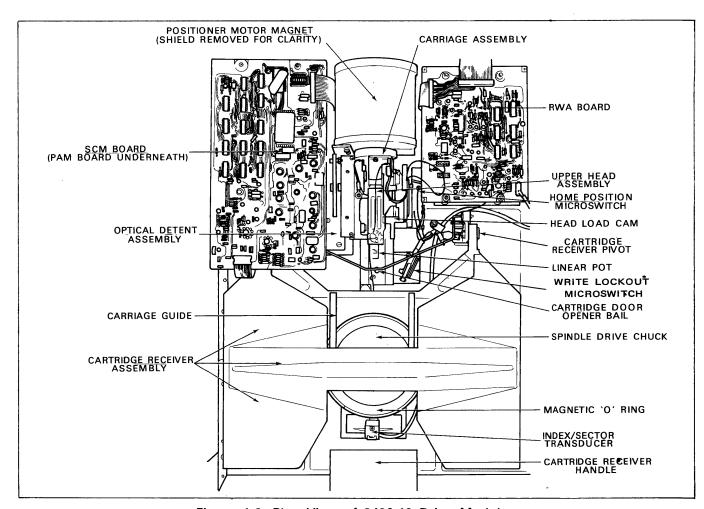
Figure 1-9. Plan View of 9480-12 Drive Module
