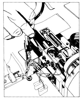
Figure 4-18. Cleaning Carriage Guide and Linear Pot
