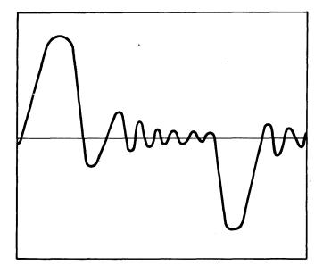
Figure 4-10b. Servo Offset Adjustment - Correct
