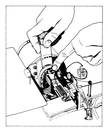
Figure 4-19. Positioner Coil Adjustment
