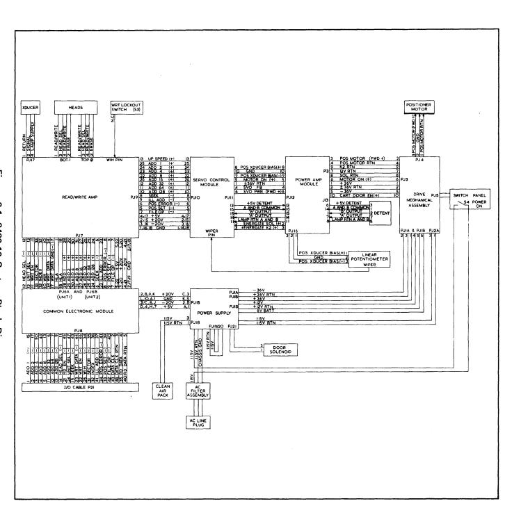
Figure 3-1. 9480-12 System Block Diagram
