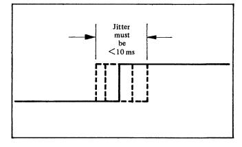
Figure 4-7. Long Servo Gate Jitter
