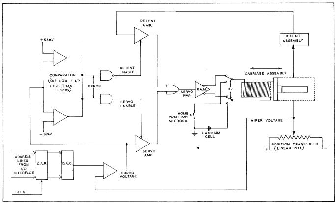
Figure 1-20. Positioning System – Coarse and Fine Servo Loops – Simplified Functional Block Diagram
