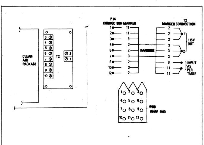
Figure 6-6. International Transformer Mounting
