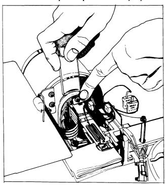
Figure 4-5. Positioner Coil Adjustment
