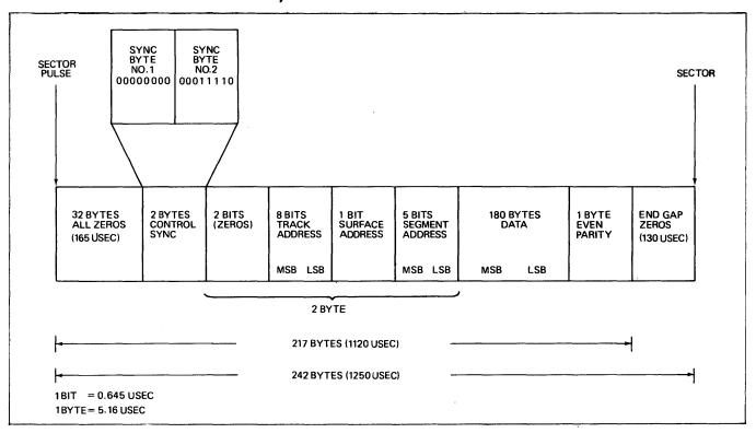
Figure 1-15. Burroughs DCD 2200 BPI 180 Byte Format
