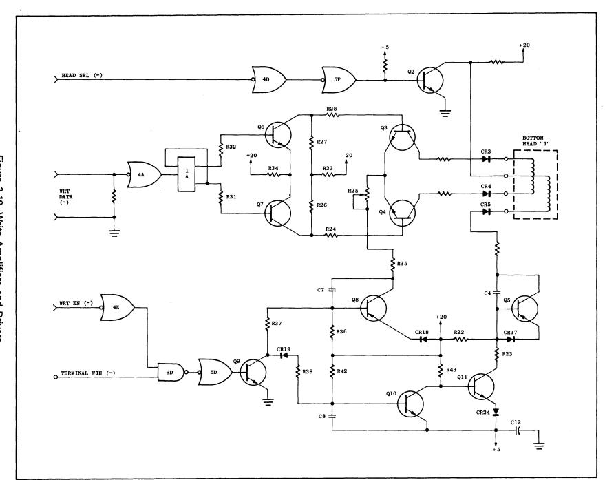
Figure 2-19. Write Amplifiers and Drivers.
