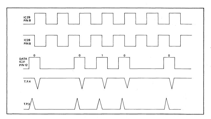
Figure 2-23. Phase-Locked Loop Timing Chart Data And Clocks Synchronized
