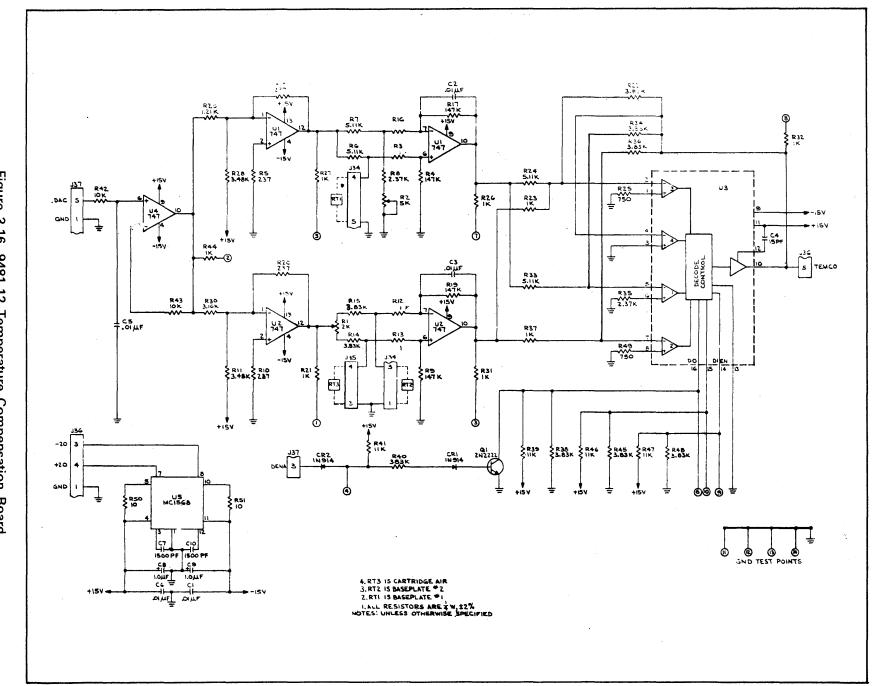
Figure 3-16. 9481-12 Temperature Compensation Board
