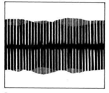
Figure 4-11b.Dibit Pattern-Head Alignment-Correct
