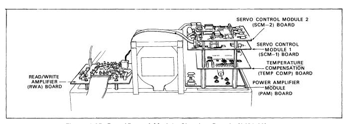
Figure 1-25. Rear View of Module Showing Boards (9481-12)
