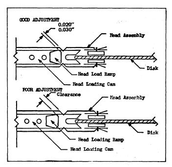
Figure 5-16. Head Load Cam Adjustment
