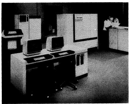
This basic B 5935 system includes a dual-display operator console with two built-in mini-disk drives for maintenance functions, a 650-lpm printer, a tape drive and controller, the central processing unit with 3.1 megabytes of main memory, and a disk drive and controller.
