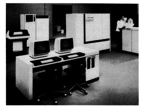
This basic B 5900 system includes a dual-display operator console with two built-in mini-disk drives for maintenance functions, a 650-lpm printer, a tape drive and controller, the central processing unit with 1.5 megabytes of main memory, and a disk drive and controller.
