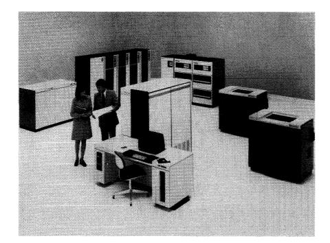
The B 1870 system is the largest member of the B 1800 family. It can have up to 524K bytes of main memory, 4.096 bytes of cache memory, and 23.6 million bytes of system disk memory.
