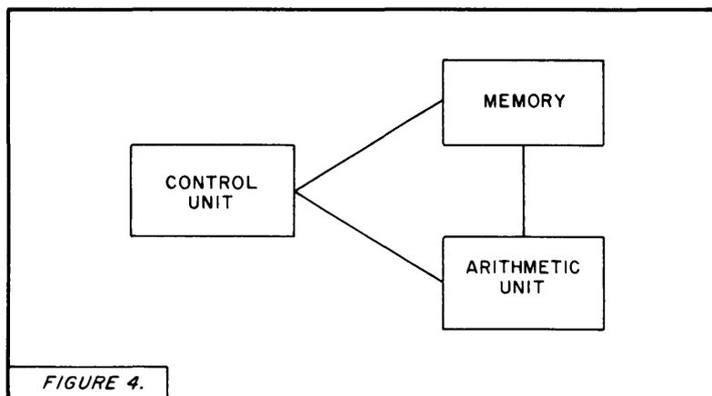
Traditionally, serial machines have demonstrated performance gains by little more than a repackaging of the basic organization of Figure 4 in faster and faster hardware. That is, computer technology has advanced from vacuum tubes to transistors to integrated circuits, with corresponding increases in the number of operations per second (tens of thousands, hundreds of thousands, and millions of operations per second respectively).
