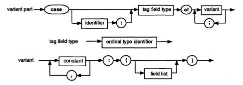
You can see from the diagram that each variant is identified by at least one constant. All constants must be distinct and of an ordinal type compatible with the tag field type. Variant and fixed fields are accessed the same way.
