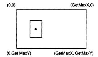
If the Boolean variable *Clip* is set to True when a call to *SetViewPort* is made, all drawings will be clipped to the current viewport. Note that the "current pointer" is never clipped. The following will not draw the complete line requested because the line will be clipped to the current viewport:
