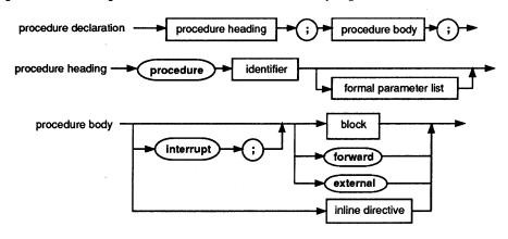
The procedure heading names the procedure's identifier and specifies the formal parameters (if any). The syntax for a formal parameter list is shown in the section "Parameters" on page 82.
