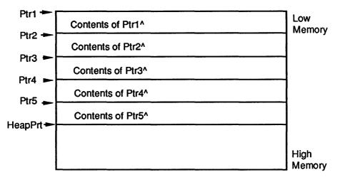
Figure 15.2: Disposal Method Using Mark and Release
