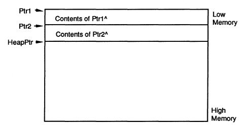
Figure 15.3: Heap Layout with Release(P) Executed
