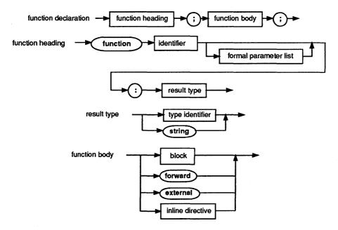
The **function** heading specifies the identifier for the function, the formal parameters (if any), and the function result type.
