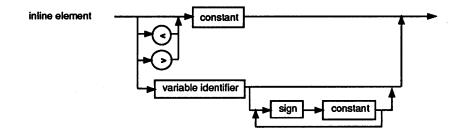
Each inline element generates 1 byte or one word of code. The value is computed from the value of the first constant or the offset of the variable identifier, to which is added or subtracted the value of each of the constants that follow it.
