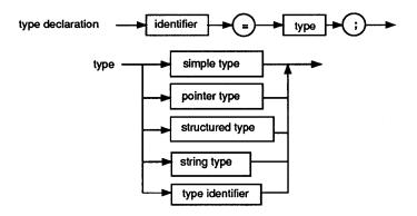
When an identifier occurs on the left side of a type declaration, it is declared as a type identifier for the block in which the type declaration occurs. A type identifier's scope does not include itself except for pointer types.
