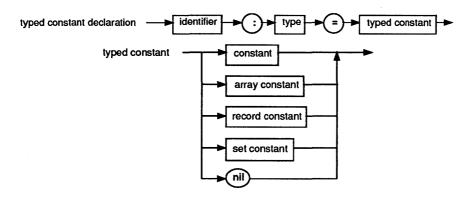
Typed constants can be used exactly like variables of the same type, and can appear on the left-hand side in an assignment statement. Note that typed constants are initialized *only once*—at the beginning of a program. Thus, for each entry to a procedure or function, the locally declared typed constants are not reinitialized.
