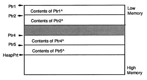
Figure 15.4: Creating a "Hole" in the Heap
