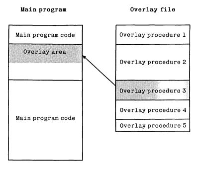
Figure 18-3: Smaller Overlay Subprogram Loaded
