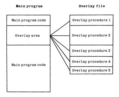
Figure 18-1 Principle of Overlay System
