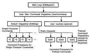
Figure 6-1. Editor Toolbox Command Dispatching: Flow of Control
