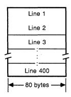
Figure 3-2. Array-of-Lines Buffer Structure
