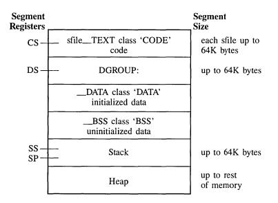
Figure 9.6: Large Model Memory Segmentation
