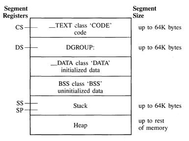
Figure 9.5: Compact Model Memory Segmentation
