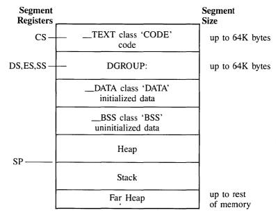
Figure 9.3: Small Model Memory Segmentation
