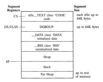
Figure 9.4: Medium Model Memory Segmentation
