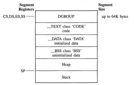
Figure 9.2: Tiny Model Memory Segmentation
