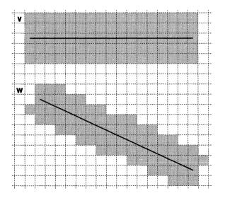
The thickness or a vertical or horizontal line can be measured in an exact number of pixels. When the line is slanted, as it is for (t) above, the stroking algorithm tries to make the line visually approximate the thickness of a vertical or horizontal line. In this way, lines retain their shape even when rotated.
