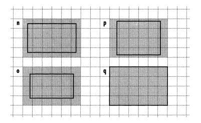
A rectangle includes every pixel that it encloses and every pixel that its sides pass through. However, as rectangle (q) illustrates, it doesn't include pixels that its sides merely touch at the boundary.
