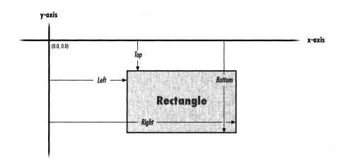
In a valid rectangle, the top y coordinate value is never greater than the bottom y coordinate, and the left x coordinate value is never greater than the right.
