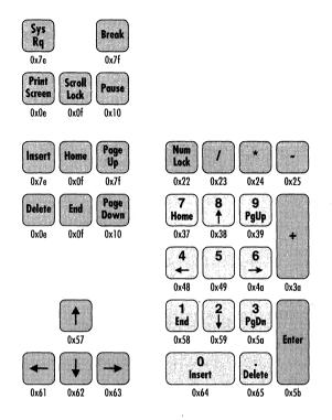
Some of the keys on a Macintosh keyboard have different labels from those shown above, but they have the same key codes. The Macintosh also adds a Power key and an "=" key on the keypad, as shown in the figure on the next page.
