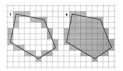
The same rules apply when stroking each segment of a polygon as would apply if that segment were an independent line. Therefore, the pen may not touch every pixel the segment passes through.
