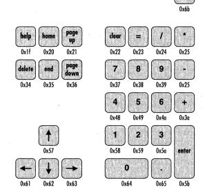
• *Modifier keys* set states that can be discerned independently of keyboard events (through the modifiers() and get\_key\_info() functions). Some modifier keys—like Caps Lock and Num Lock—toggle in and out of a locked modifier state. Others—like Shift and Control—set the state only while the key is being held down.
