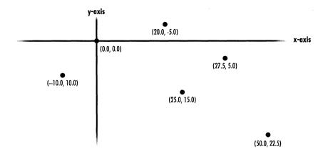
*y*-coordinate values are greater towards the bottom of the display and smaller towards the top, *x*-coordinate values are greater to the right and smaller to the left.
