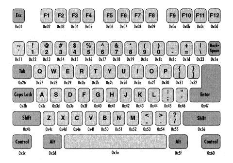
Different keyboards locate keys in slightly different positions. The function keys may be to the left of the main keyboard, for example, rather than along the top. The backslash key (0x33) shows up in various places—sometimes above the Enter key, sometimes next to Shift, and sometimes in the top row (as shown here). No matter where these keys are located, they have the codes indicated in the illustration above.
