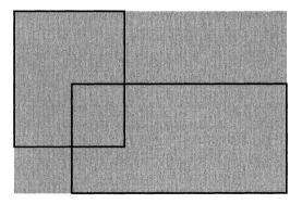
The union is computed by selecting the smallest left and top coordinate values from the two rectangles, and the greatest right and bottom coordinate values. In the following example,
