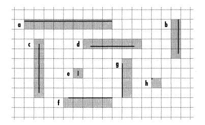
Only pixels that the line path actually passes through are colored to display the line. If a path begins or ends on a pixel boundary, as it does for examples (a) and (b) in the illustration, the pixels at the boundary aren't colored unless the path crosses into the pixel. The pen touches the fewest possible number of pixels.
