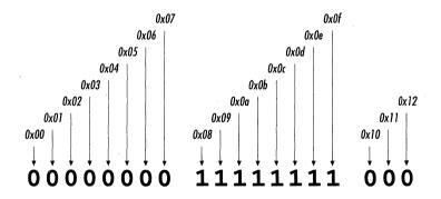
Bit numbers start with 0 and match key codes. For example, bit  $0x_3c$  corresponds to the *A* key,  $0x_3d$  to the *S* key,  $0x_3e$  to the *D* key, and so on. The first bit is  $0x_00$ , which doesn't correspond to any key. The first meaningful bit is  $0x_01$ , which corresponds to the Escape key.
