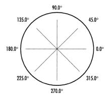
For example, if *angle* is  $180.0^{\circ}$  and *span* is  $90.0^{\circ}$ , the arc would be the lower left quarter of the ellipse. The same arc would be drawn if *angle* were  $270.0^{\circ}$  and *span* were  $-90.0^{\circ}$ .
