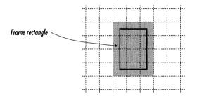
Since the pixels on the edges of this  $2.0 \times 3.0$  rectangle are treated as being inside the rectangle, the view covers a 3 pixel  $\times$  4 pixel area.
