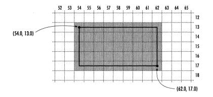
Because the BRect structure is a basic data type for graphic operations, it's constructed more simply than most other Interface Kit classes: All its data members are publicly accessible, it doesn't have virtual functions, and it doesn't inherit from BArchivable or any other class. Within the Interface Kit, BRect objects are passed and returned by value.
