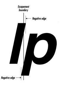
Note that the italic "l" extends beyond its escapement to the right, and that the "p" begins before its escapement to the left. In this case, instead of separating the adjacent characters, the edges determine how much they overlap.
