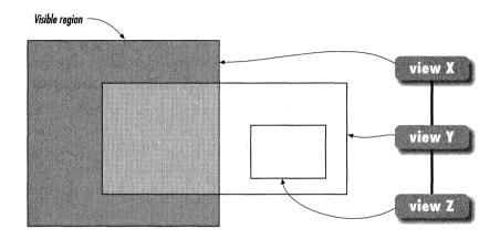
The visible region of a view might be further restricted if its window is obscured by another window or if the window it's in lies partially off-screen. The visible region includes only those areas that are actually visible to the user. For example, if the three views in the previous illustration were in a window that was partially blocked by another, their visible regions might be much smaller, as shown in the next figure:
