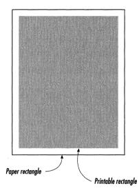
Both rectangles are stated in a coordinate system that has its origin at the left top corner of the page. Thus, the left and top sides of the rectangle returned by PaperRect() are always 0.0. PrintableRect() locates the printable rectangle on the paper rectangle. However, DrawView() assumes coordinates that are local to the printable rectangle—that is, an origin at the left top corner of the printable rectangle rather than the paper rectangle.
