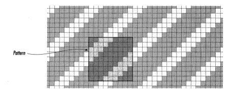
The dotted lines in this illustration show the separation of the screen into pixels. The thicker black line outlines one  $8 \times 8$  square that the pattern defines.
