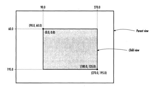
When a view moves to a new location in its parent, its frame rectangle changes but not its bounds rectangle. When a view scrolls its contents, its bounds rectangle changes, but not its frame. The frame rectangle positions the view in the world outside; the bounds rectangle positions the contents inside the view.
