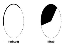
The arc is a section of the ellipse inscribed in *rect*—or the ellipse located at *center*, where the horizontal distance from the center to the edge of the ellipse is measured by *xRadius* and the vertical distance from the center to the edge is measured by *yRadius*.
