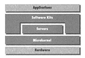
The API for all system software is organized into several "kits." Each kit has a distinct domain—there's a kit that contains the fundamental software for creating and running an application, a kit for putting together a user interface, one for accessing the file system, another for networking, and so on.
