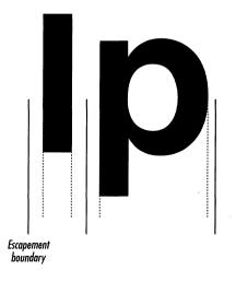
This is the normal case. The left edge is a positive value measured rightward from the left escapement boundary. The right edge is a negative value measured leftward from the right escapement boundary.
