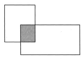
The intersection is computed by taking the greatest left and top coordinate values of the two rectangles, and the smallest right and bottom values. In the following example,
