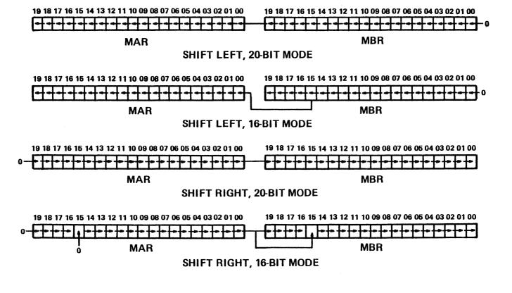
Figure 2.3: Shifting Picture 7 2.10 Loading and Reading Microcode
