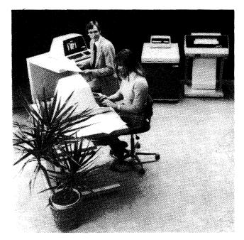
The Basic Four System 210 is an information processing system designed for the first-time user. The 210's base configuration includes 64K-bytes of main memory, a 10M-bytes fixed disk system, a 9.2M-bytes magnetic tape cartridge drive, a video display terminal, and a bidirectional 80 characters-per-second matrix printer. DataWord 11 word processing hardware/software is available for Systems 210, 510, 610 and 730.
