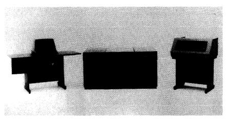
The Basic Four System 610 supports from 64K to 256K bytes of main memory, from 35 to 300 million bytes of disk storage, and up to 16 video data terminals. A basic system with 64K bytes of memory, 35 million bytes of disk storage, one VDT, and a 150-lpm printer sells for \$51,400.
