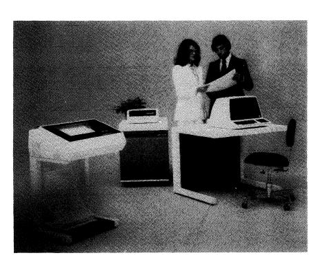
The basic System 200, the entry-level member of the Basic Four line, consists of a CPU with 32K bytes of memory, one 10-megabyte disk unit, one video display terminal, a 120-cps printer, and a 2.5-megabyte magnetic tape cartridge unit. The purchase price for this configuration is \$29,000. A System 200 can be expanded to include up to 40K bytes of memory, 20 megabytes of disk storage, and two VDTs
