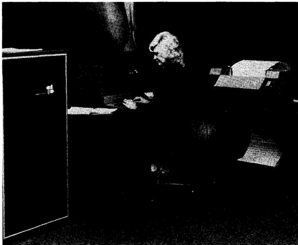
*Shown here is the Basic/Four Model 350, which includes a central processing unit with 8K bytes of core memory, a low-capacity disc drive containing 2.1 million bytes, a medium-speed matrix printer, and a video display terminal including desk. The base purchase price of the system is \$32,400.*
