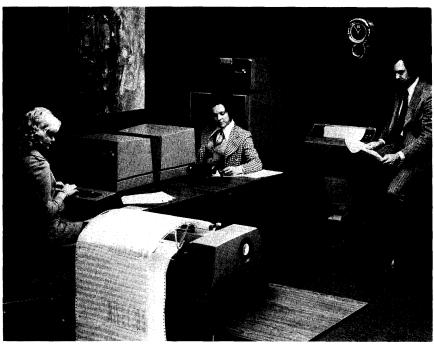
Shown here is the Basic/Four Model 400 which includes a central processor with 16K bytes of core memory, a high capacity disc drive containing 4.2 million bytes, an industry-compatible magnetic tape unit, two printer units, and two CRT operator stations.
