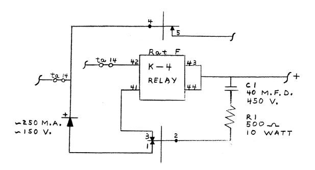
With the Flexowriter modified as shown above nine (9) to eleven (11) tape feed holes will automatically be punched on the tape following each character typed on the keyboard. The tape can then be read into the computer one character at a time under program control.
