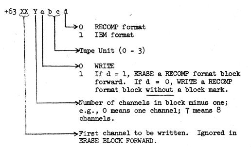
For example, to WRITE a 3-channel block from channels 55, 56 and 57 in RECOMP format on tape unit 3, use the following command:
