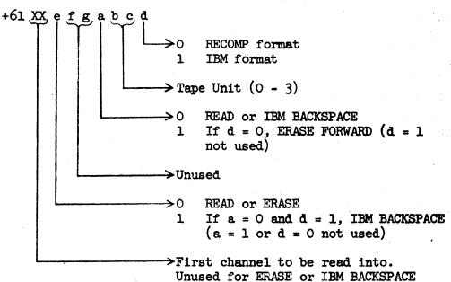
For example, to read an IBM block into Channel 55 (and succeeding channels, if needed) from tape unit 2, use the following command:
