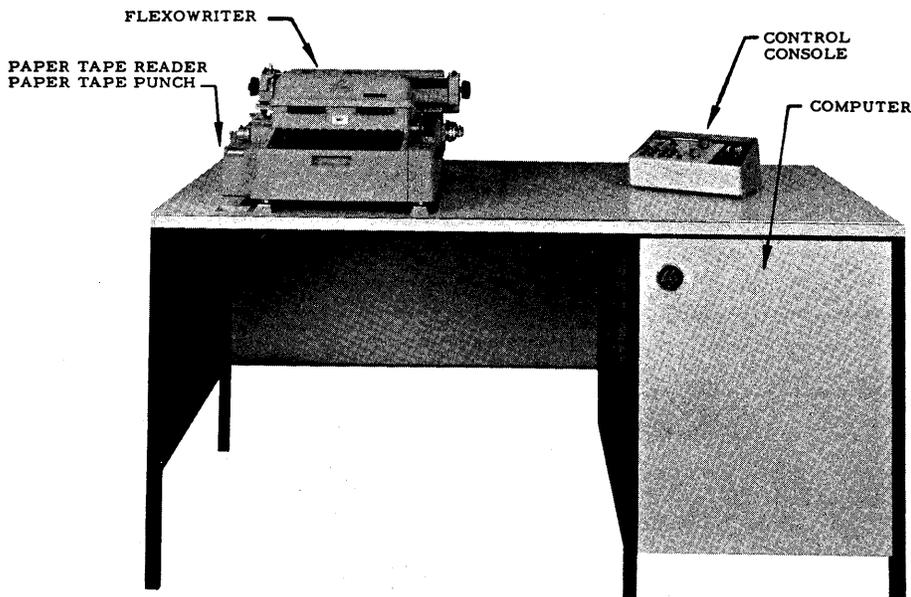
Figure 1. RECOMP III Computer Components
