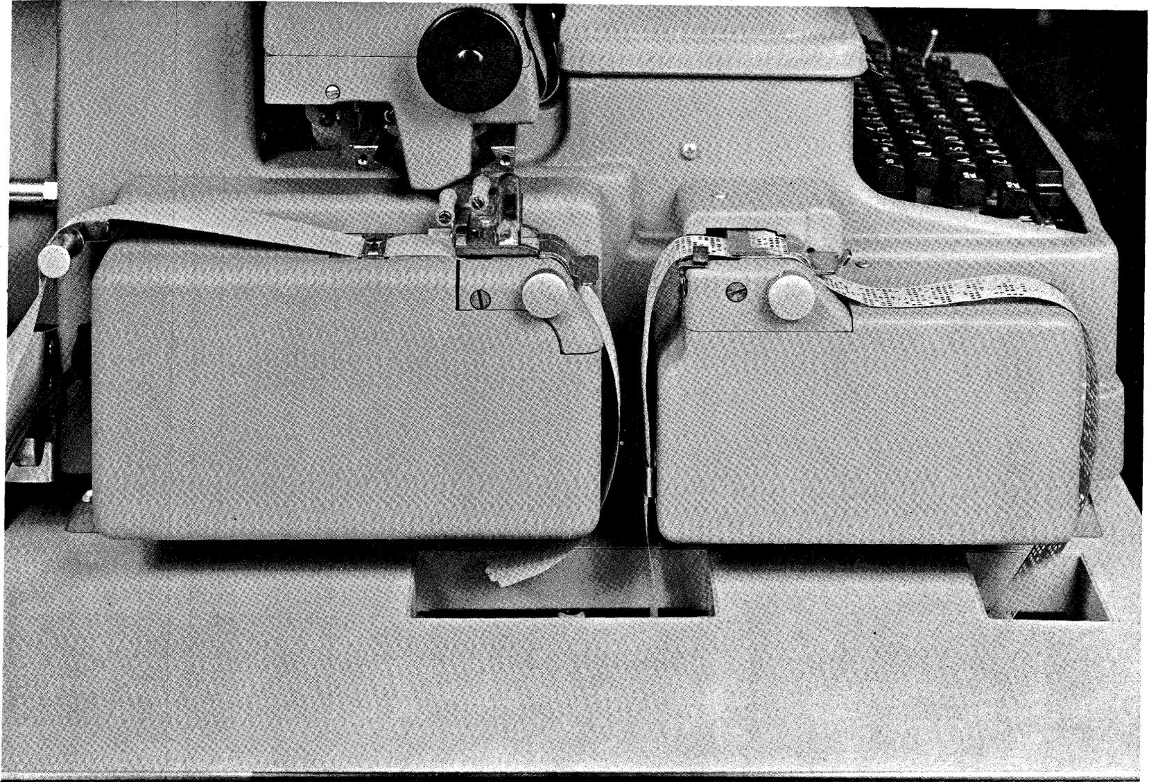
Figure 4. Flexowriter Tape Punch and Tape Reader
