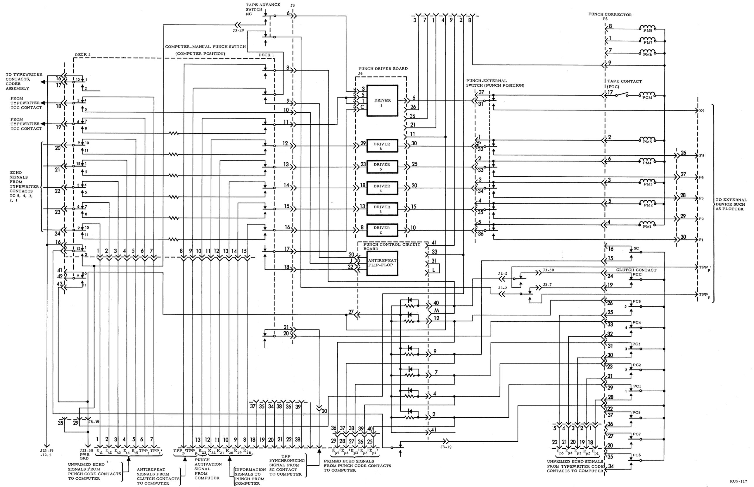
Figure 48. Punch Input-Output Schematic
