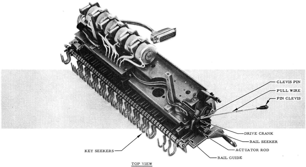
Figure 23. Decoder Assembly
