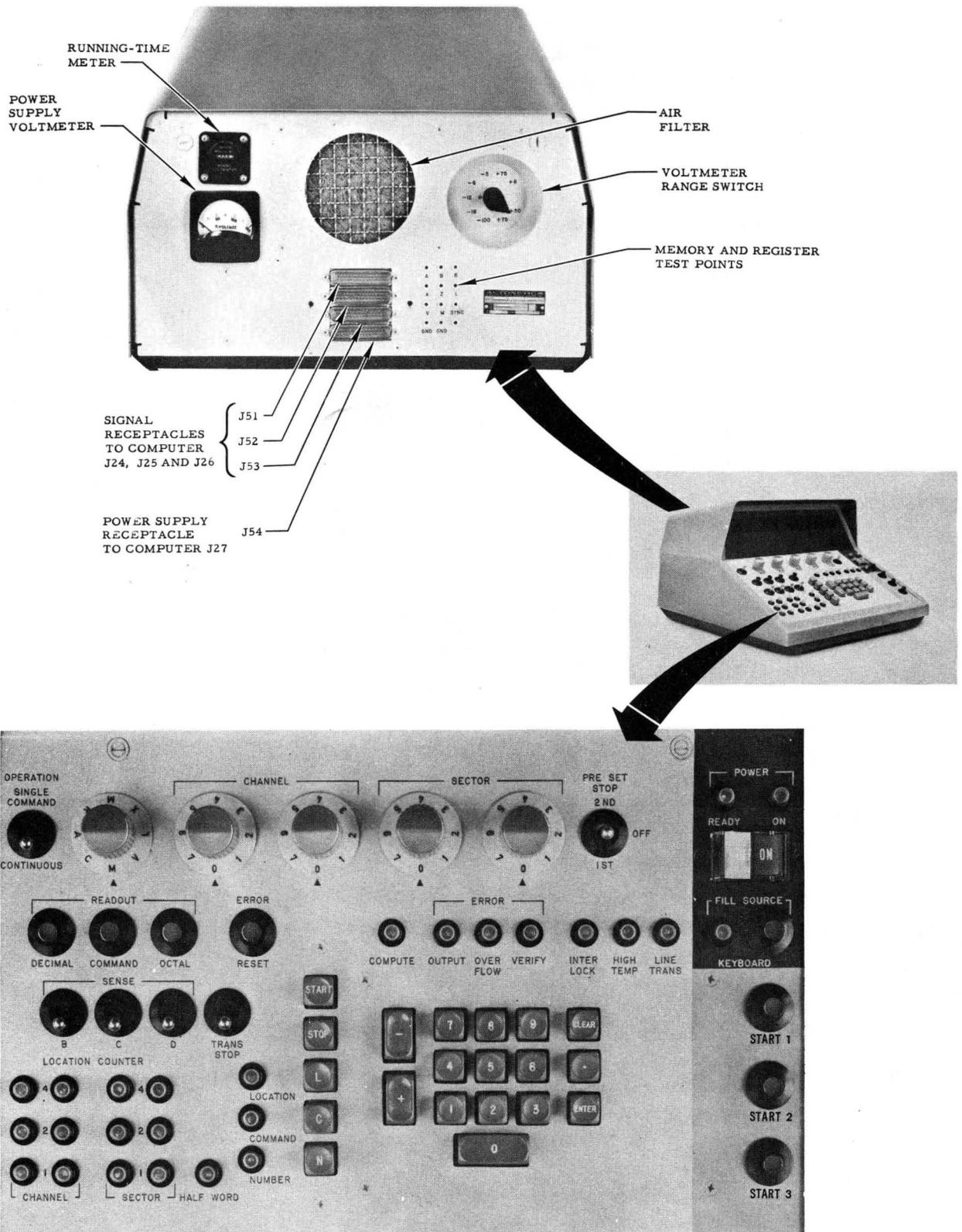
Figure 10. Control Console, Front and Rear Views
