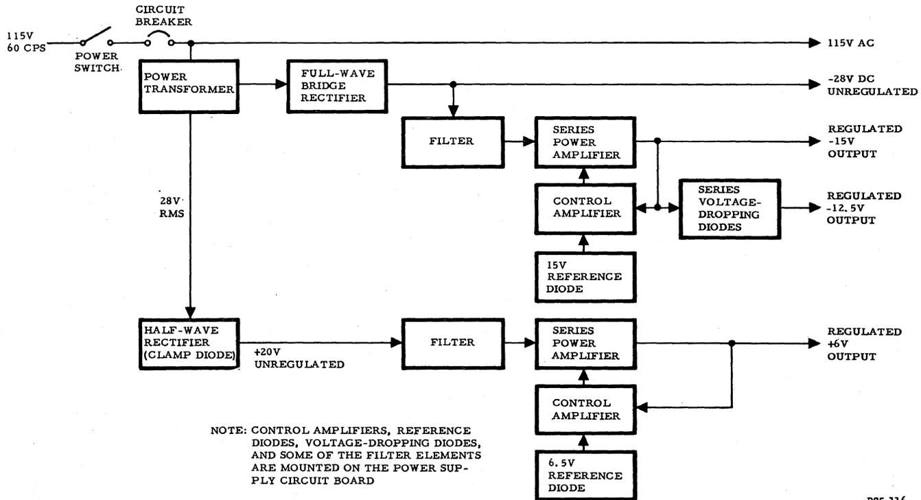
Figure 51. Tape Punch Power Supply (Block Diagram)
