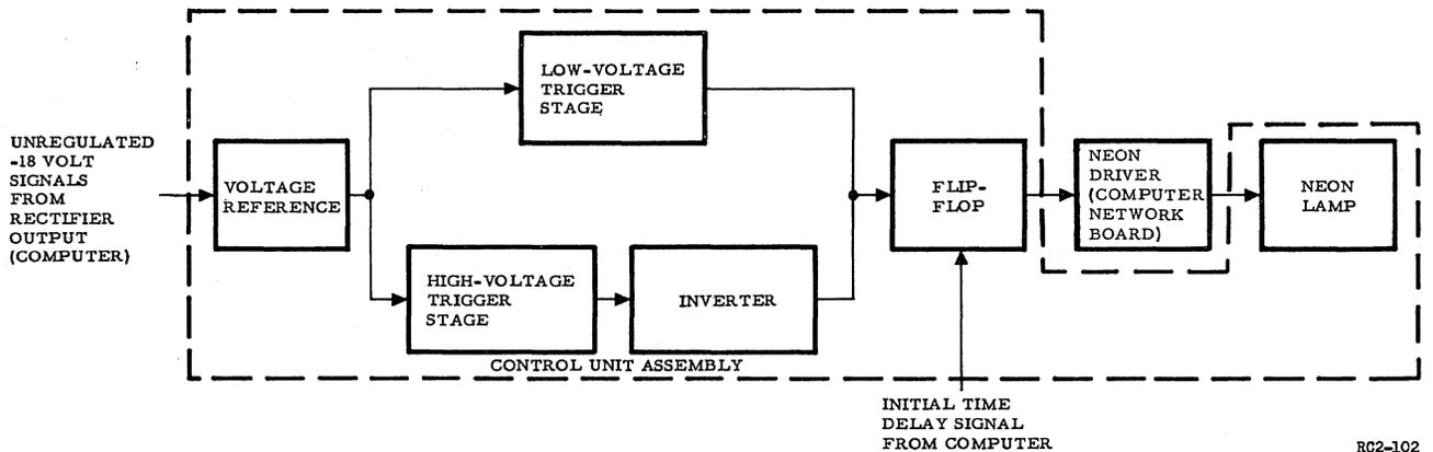
Figure 14. Voltage Transient Trigger Diagram
