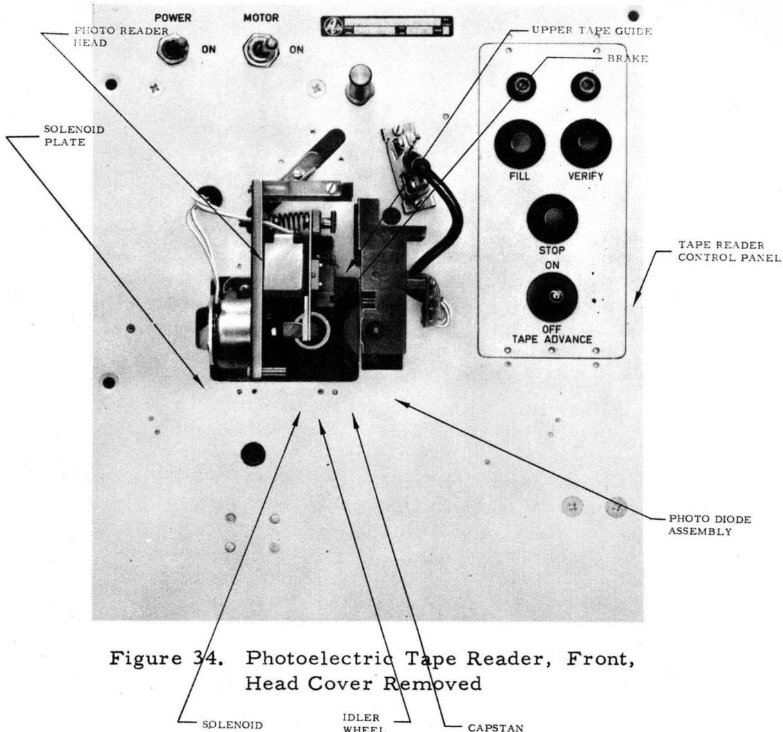
Figure 34. Photoelectric Tape Reader, Front, Head Cover Removed
