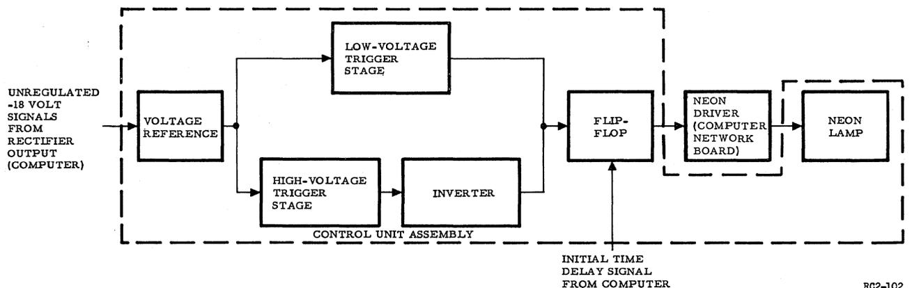
Figure 14. Voltage Transient Trigger Diagram
