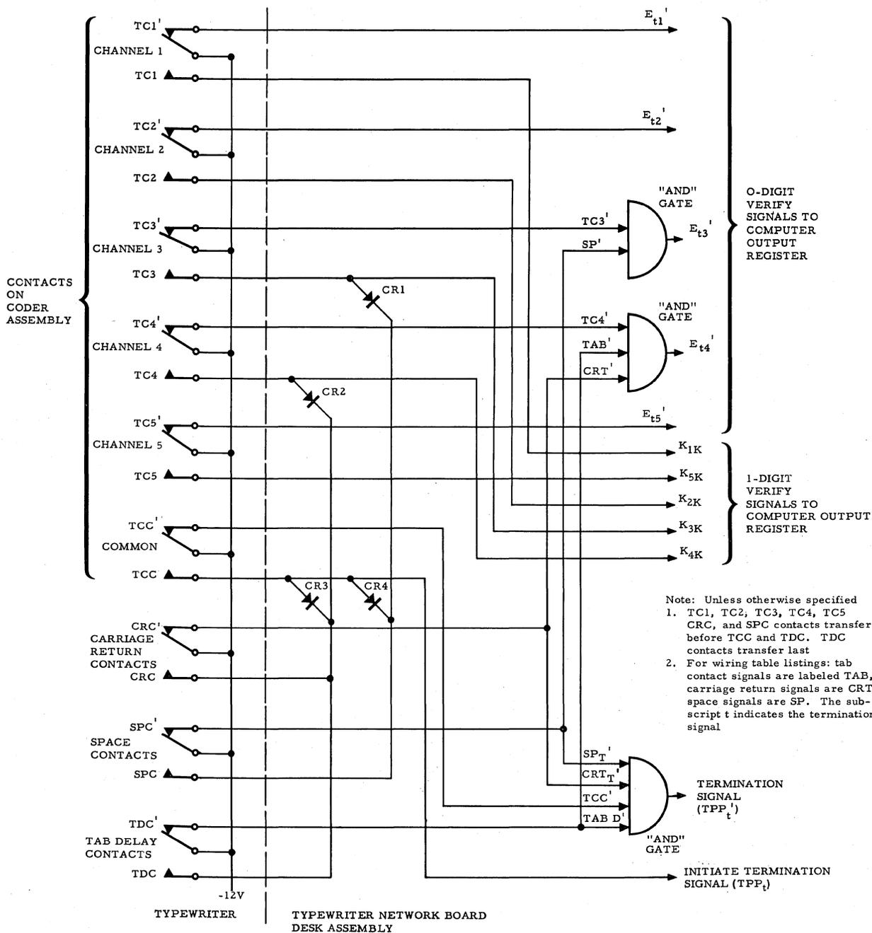
Figure 25. Typewriter Coding, Simplified Diagram
