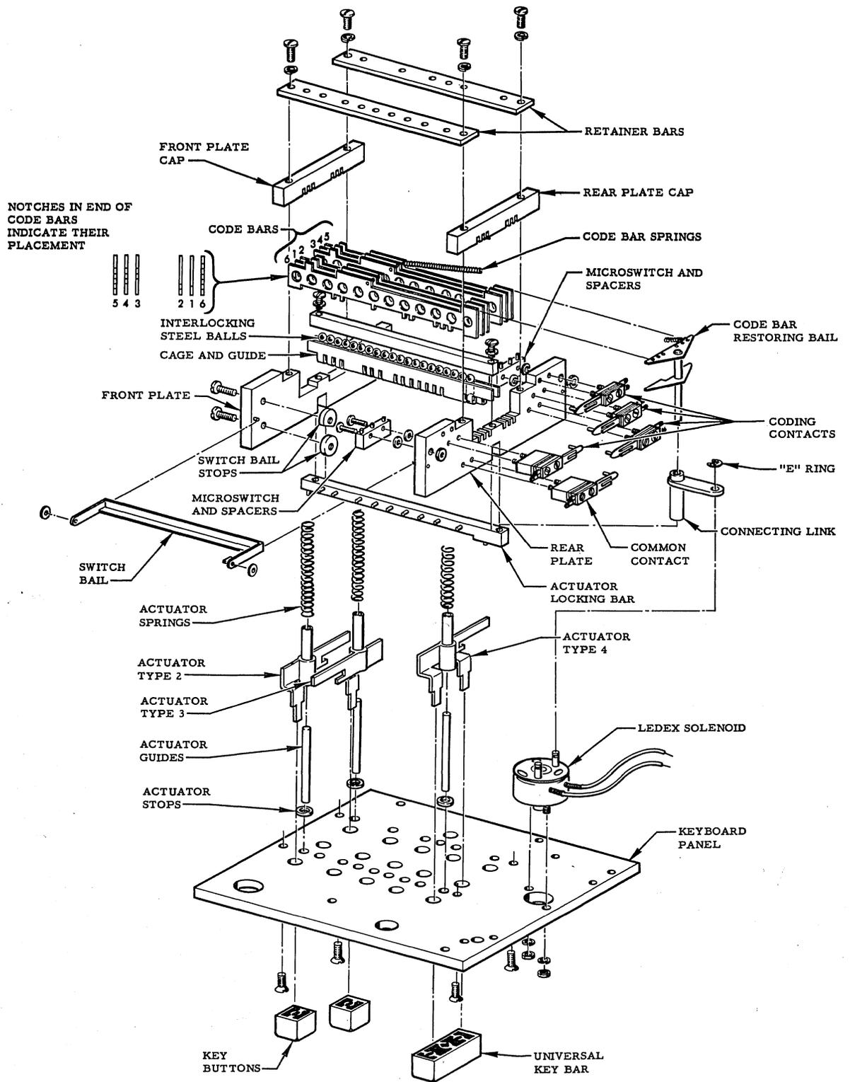
Figure 16. Control Console Keyboard, Exploded View
