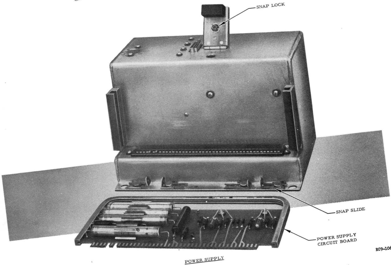
Figure 32. Control Chassis and Power Supply Disassembled
