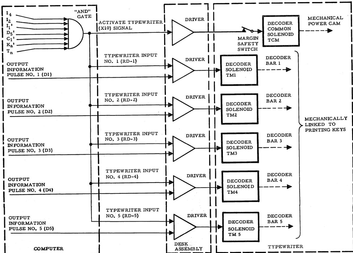
Figure 22. Typewriter-Decoding Block Diagram
