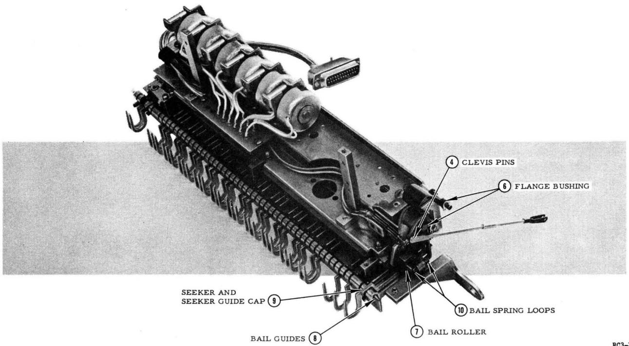
Figure 29. Decoder Lubrication Points
