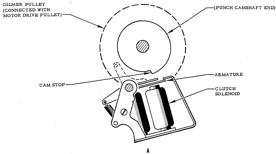
A. CAM SHAFT ACTUATION
