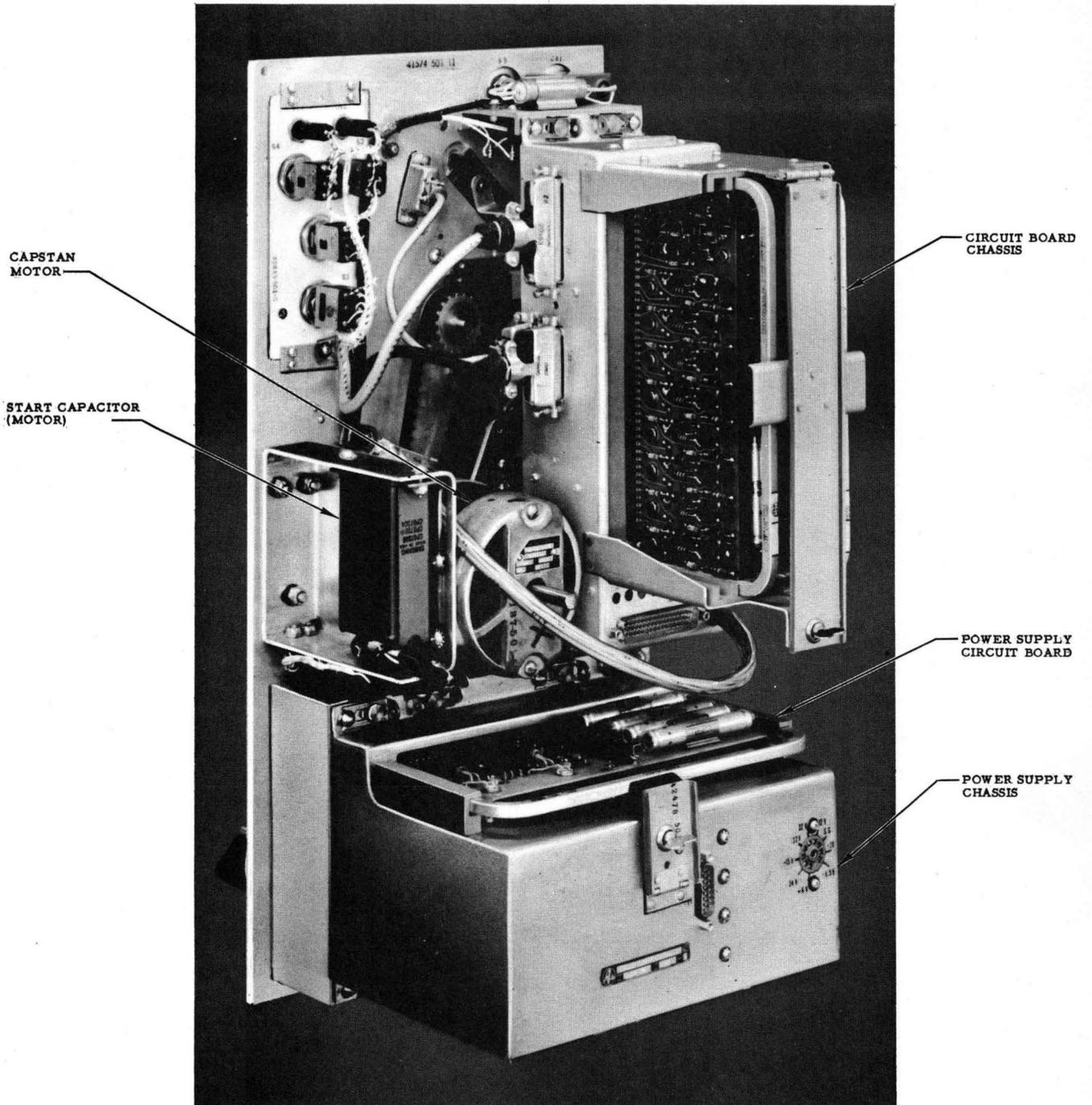
Figure 36. Photoelectric Tape Reader, Rear
