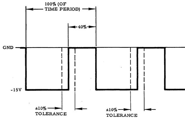
a. CLOCK (SPROCKET HOLE) CHANNEL OUTPUT
