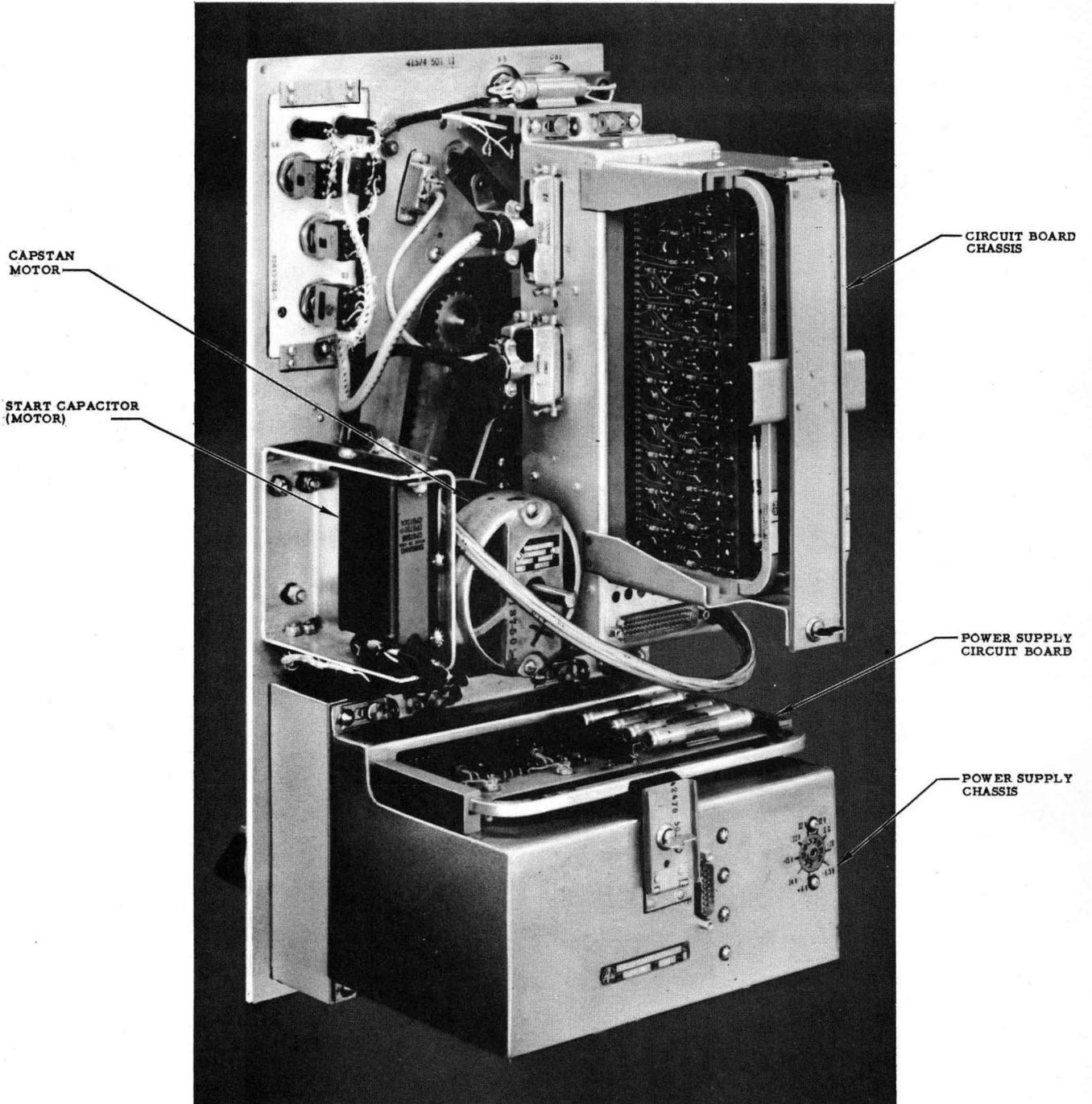
Figure 36. Photoelectric Tape Reader, Rear
