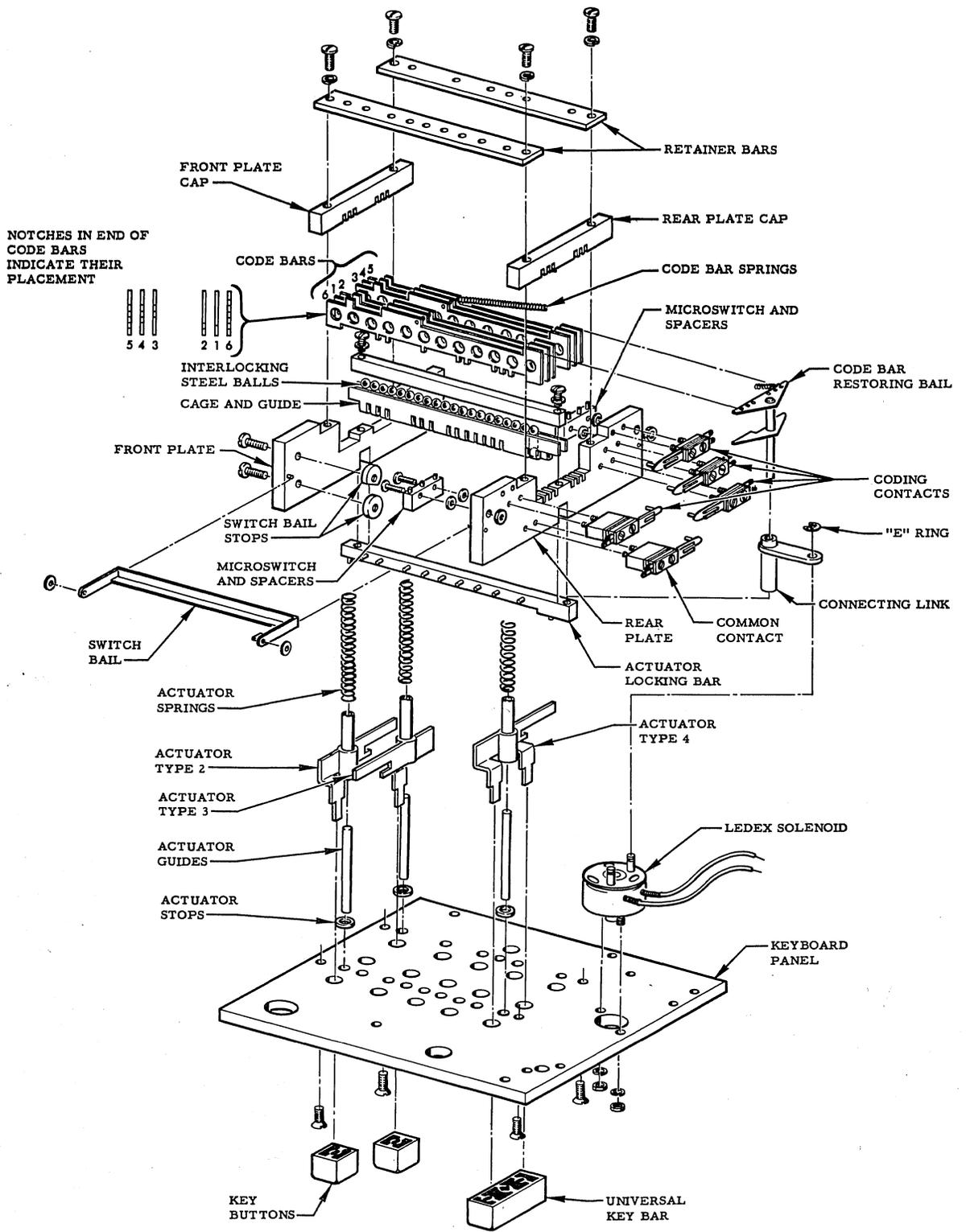
Figure 16. Control Console Keyboard, Exploded View
