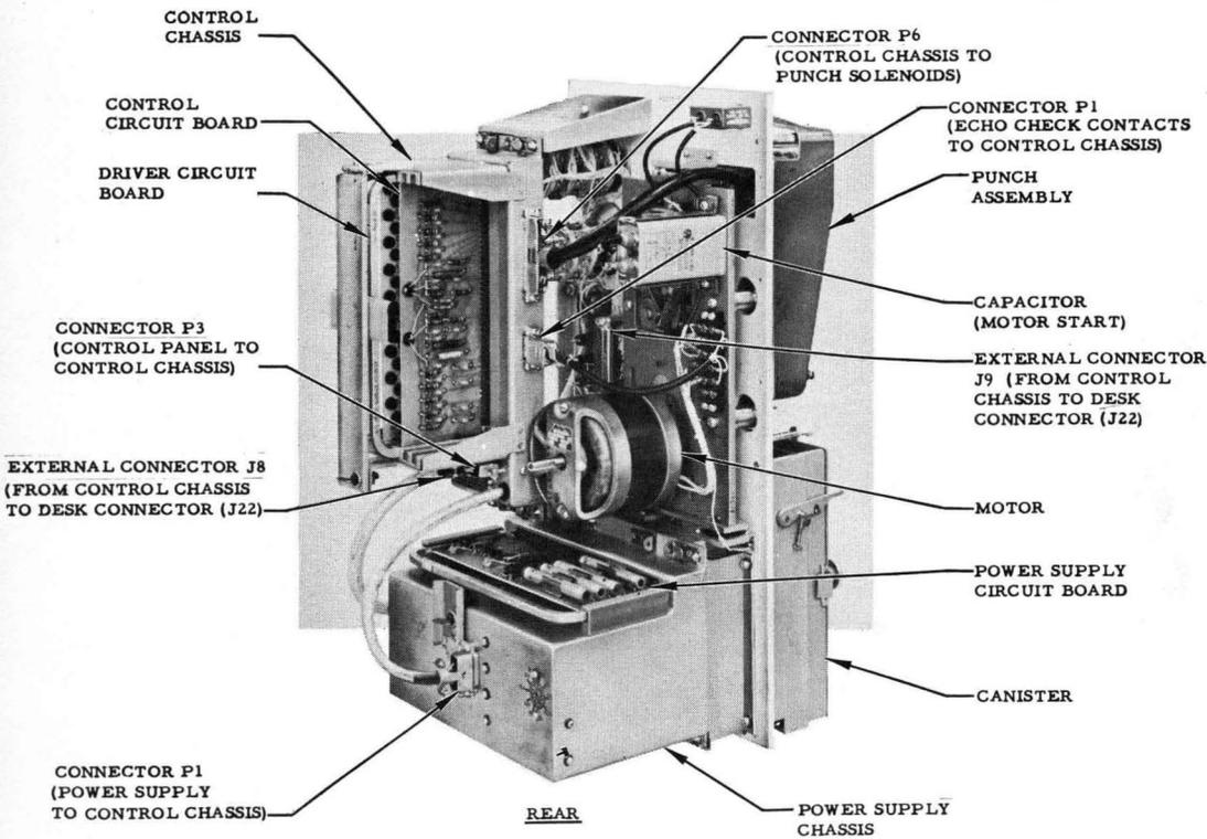
Figure 44. Tape Punch Recorder Interior View
