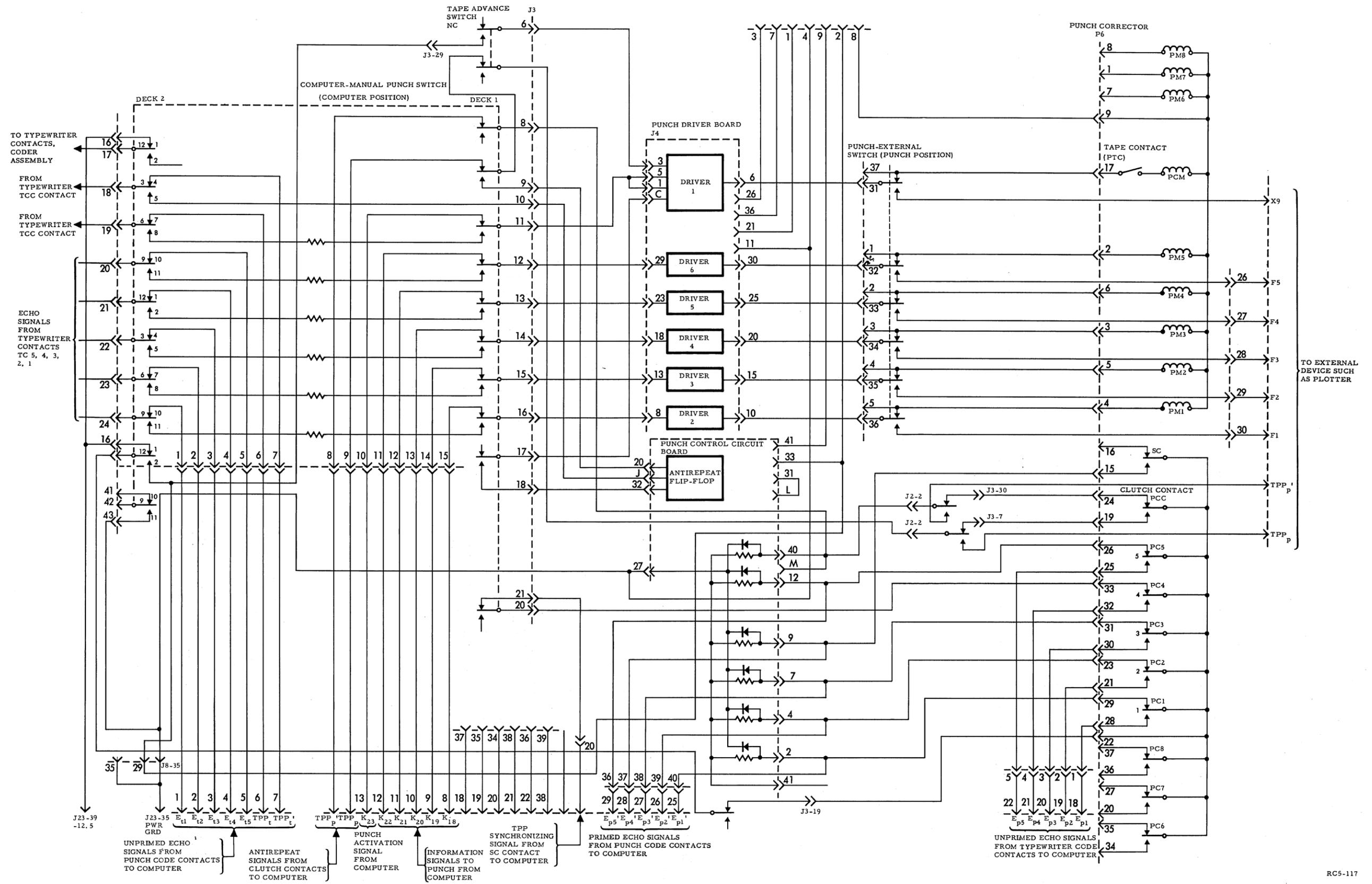
Figure 48. Punch Input-Output Schematic
