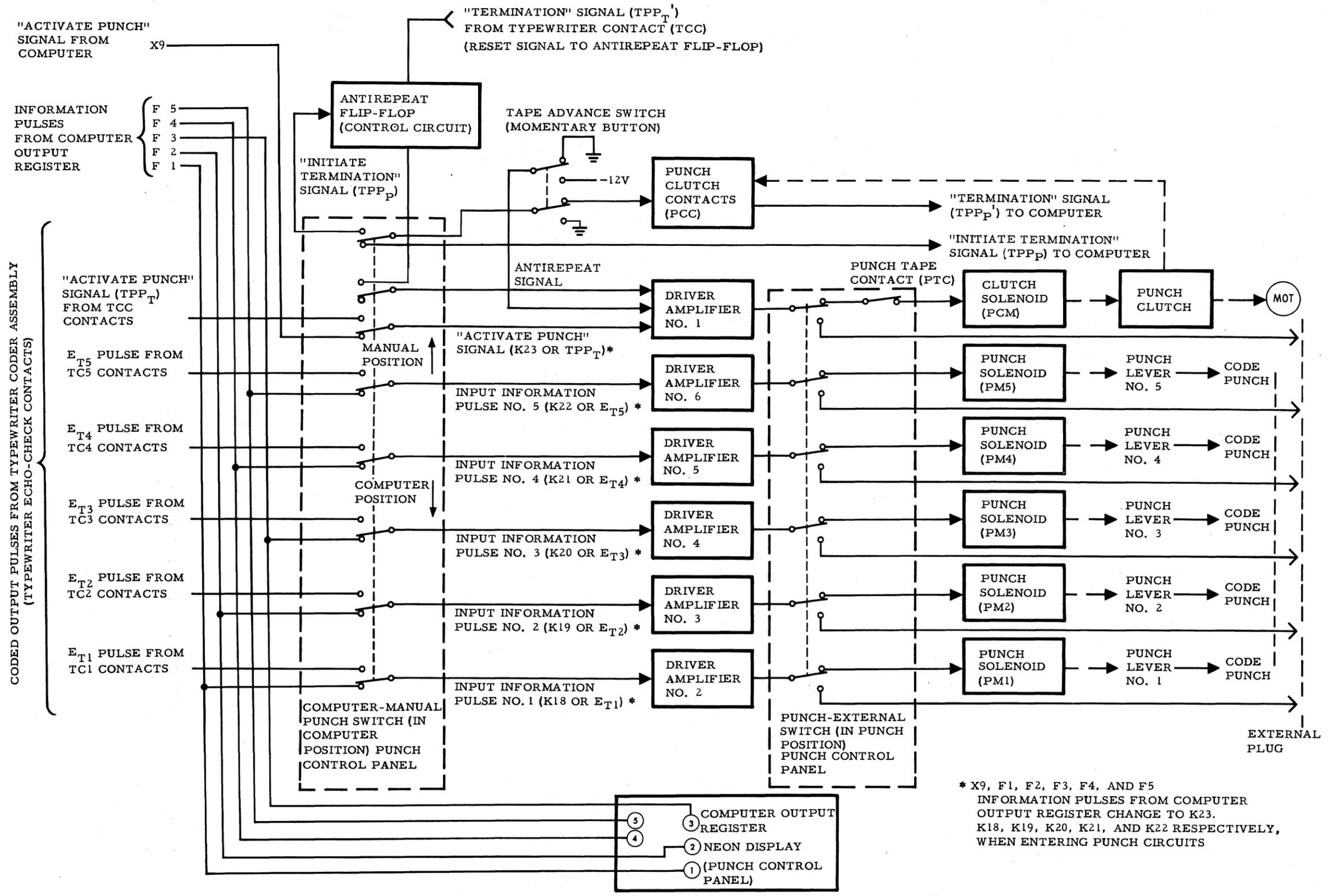
Figure 47. Tape Punch Activation Block Diagram
