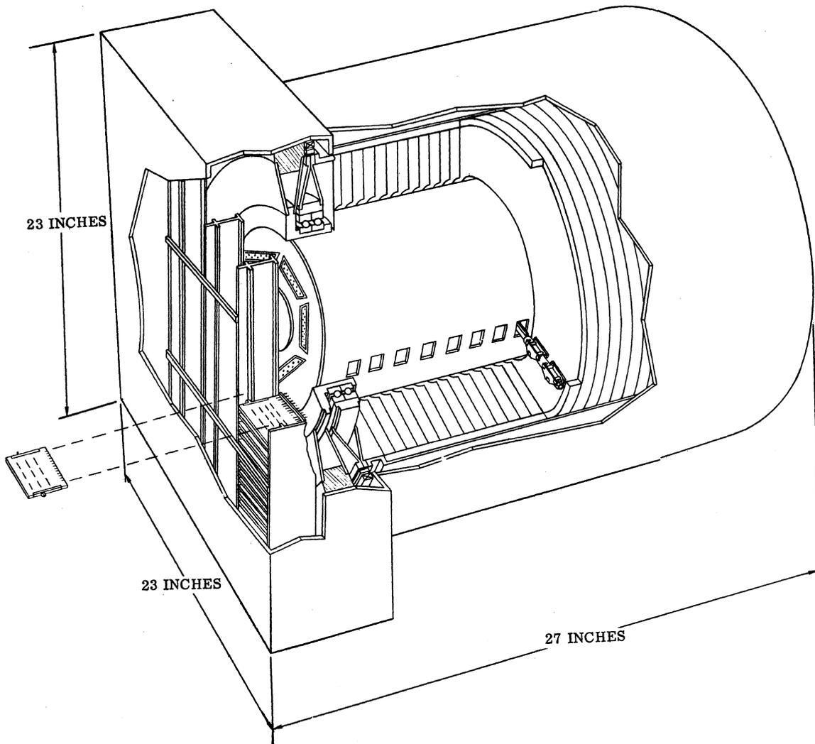
Figure 3. One-Gigabit Digital Disk File
