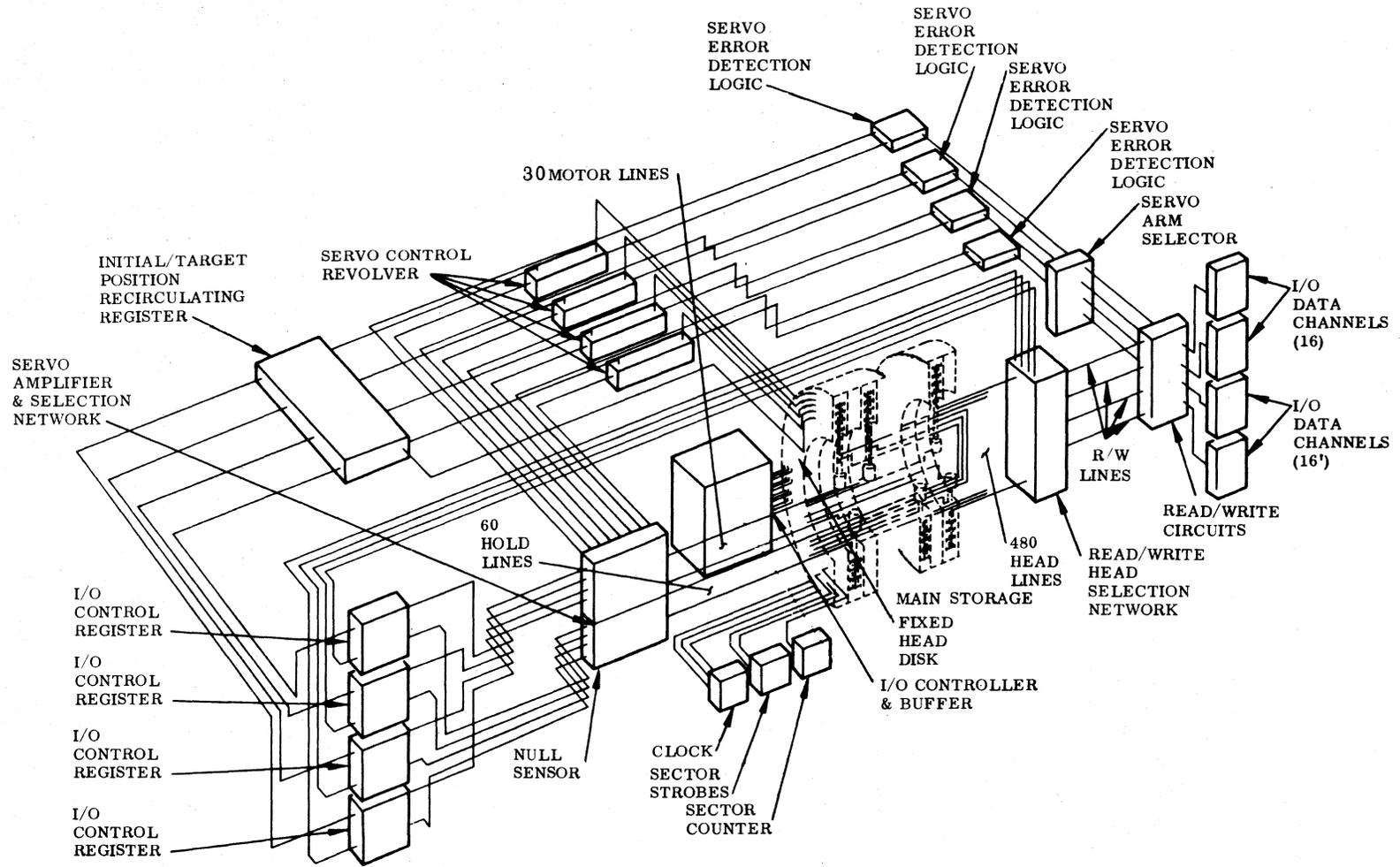
Figure 2. Functional Schematic of 30-Arm Digital Disk File
