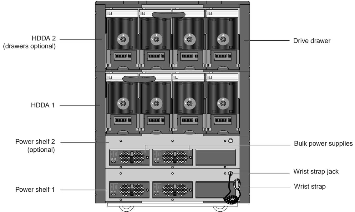
**Figure 1. NS 7000/030 storage subsystem (front view)**
