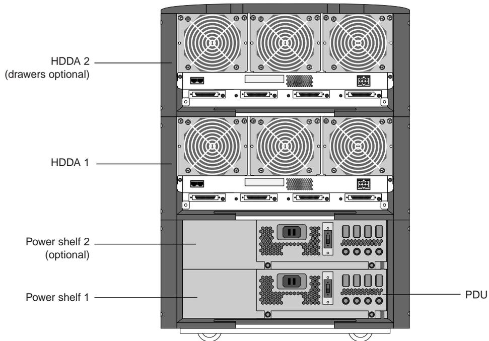
**Figure 2. NS 7000/030 storage subsystem (back view)**
