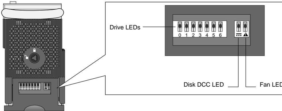
**Figure 32. Disk DCC LED (drive drawer front panel)**
