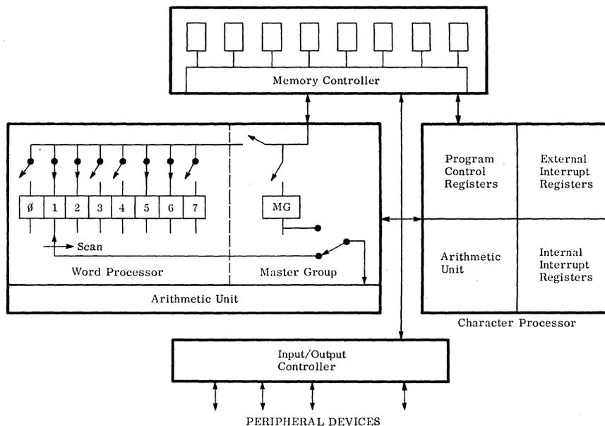
Figure 1. Logical Diagram of the Principal Components of the Honeywell Model 8200.
