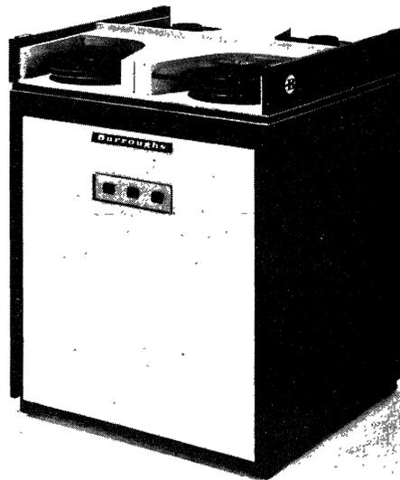
This Clustered Magnetic Tape Unit contains four independent tape transports (Section 210:092).
