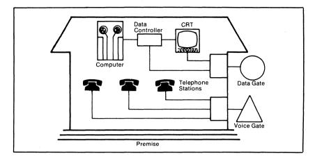
Figure 8-3. Separate Voice and Data Gates
