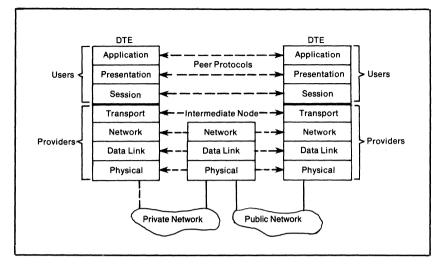
Figure 9-3. Layered Architecture
