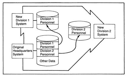
Figure 4-3. Partitioning an Existing Data Base
