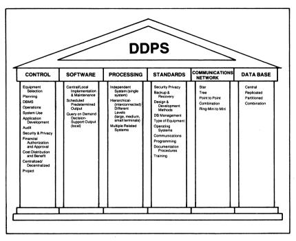
Figure 1-1. The Six Elements of Distributed Data Processing Systems
