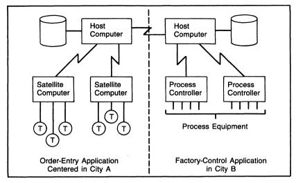
Figure 7-1. Loosely Coupled Applications
