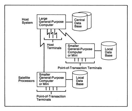
Figure 4-1. Host/Satellite Distributed Processing
