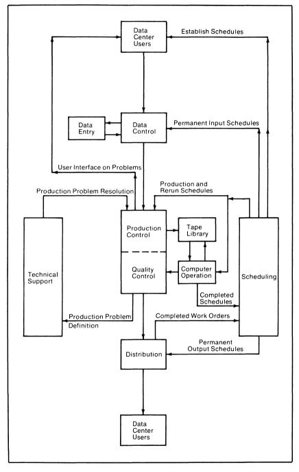
Figure 4-1. Typical Data Center Work Flow
