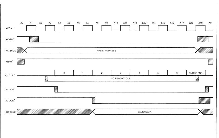
Figure 4 CPU non-LANCE Read-Timing Diagram
