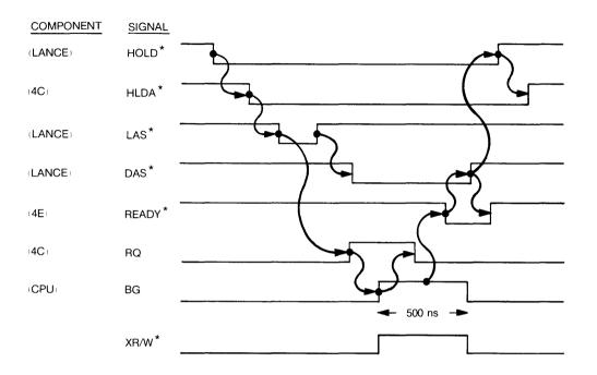
Figure 3 Expansion Board Cycle Diagram
