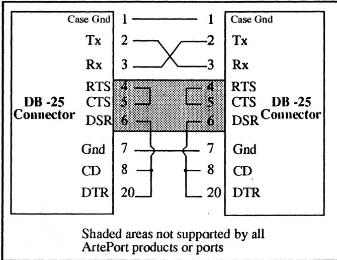
Figure 3-5. Null Modem Cable
