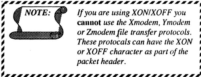
XON/XOFF are two control characters that are a holdover from the old Teletype days. They are used to control data being sent by the computer. The modem will send the XOFF character to indicate that it can not handle any more data. When it's able to handle additional data, it will send an XON character.
