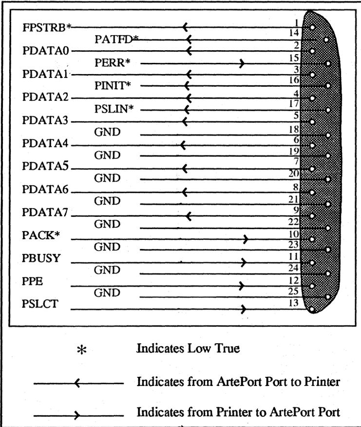
Figure 3-8. Parallel DB-25 Connector
