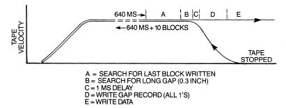
Figure 9-28 Tape motion, Write-Reposition Sequence.
