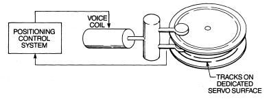
Figure 2-5 Closed-loop with dedicated servo surface.
