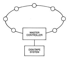
Figure 1-21 Loop-type network with shared mass storage.
