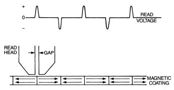
Figure 1-11 Read pulses generated by flux reversals.
