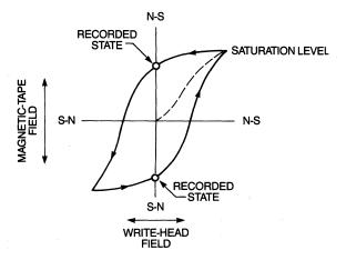
Figure 1-13 Conventional saturated recording.
