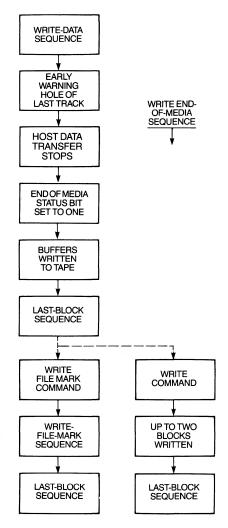
Figure 9-24 Write End-of-Media Sequence.
