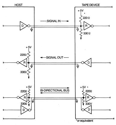
Figure 9-8 Interface drivers and receivers.
