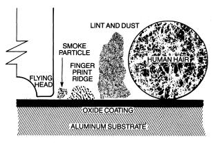
Figure 2-2 Sources of disk contamination.
