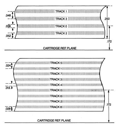
Figure 9-4 Track dimensions, <sup>1</sup>/<sub>4</sub>-inch cartridge tape.
