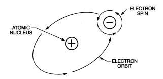
Figure 1-8 Electron spin as a source of magnetic force.
