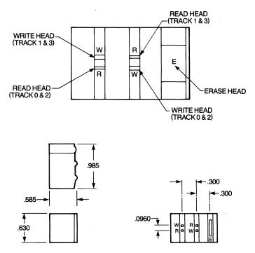
Figure 9-5 Read-after-write head dimensions.
