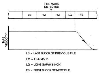
Figure 9-34 Tape motion, Read-File-Mark Sequence.
