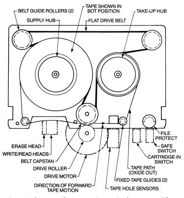
Figure 5-4 Internal construction, <sup>1</sup>/<sub>4</sub>-inch tape cartridge.
