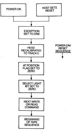
Figure 9-12 Power On/Reset Sequence.
