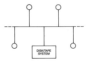
Figure 1-23 Bus-type network with shared mass storage.
