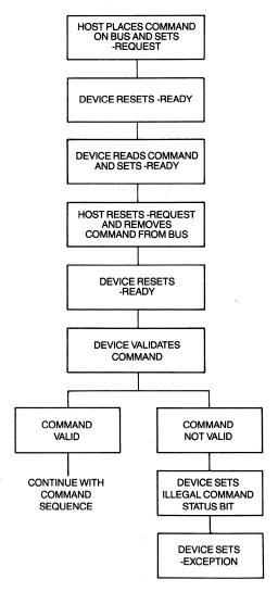
Figure 9-13 Command-Reject Sequence
