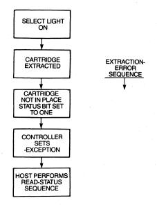
Figure 9-14 Cartridge-Extraction Sequence.
