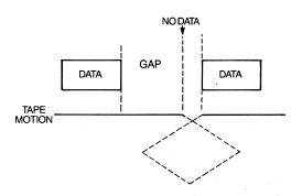
Figure 4-6 Interrupted streaming, ½-inch tape.
