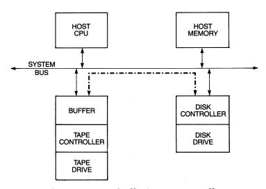
Figure 7-3 Data buffer in tape controller.
