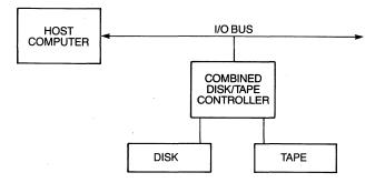
Figure 1-19 Combined disk-tape mass storage system.
