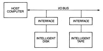
Figure 1-18 Intelligent devices with separate host interfaces.
