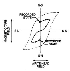
Figure 1-14 Unsaturated recording for higher densities.
