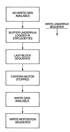
Figure 9-22 Write-Underrun Sequence.
