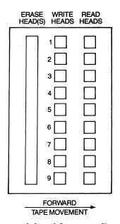
Figure 4-1 Nine-track head for recording on <sup>1</sup>/<sub>2</sub>-inch tape.
