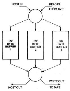
Figure 5-19 Three-block buffer for write and read operations.
