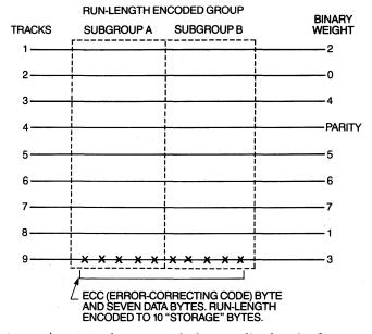
Figure 4-3 GCR (group-coded recording) ½-inch tape.
