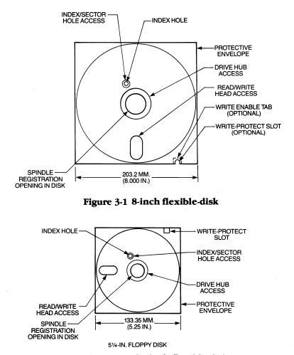
Figure 3-2 5<sup>1</sup>/<sub>4</sub>-inch flexible disk
