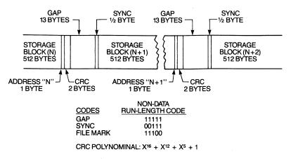
Figure 5-16 Streaming-cartridge tape format.
