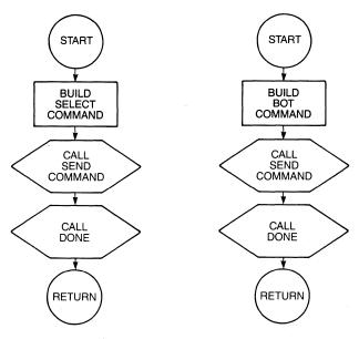
Figure 6-5 Flow diagrams, SELECT and BEGINNING OF TAPE commands.
