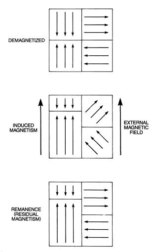
Figure 1-9 Magnetism as a function of domain size.
