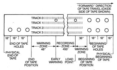
Figure 5-7 Tape-position holes, <sup>1</sup>/<sub>4</sub>-inch cartridge tape.
