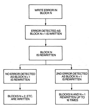
Figure 9-30 Write-Error Sequence.
