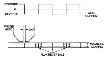
Figure 1-10 Flux reversals produced by write current.
