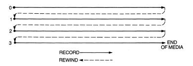
Figure 5-8 Four-track, forward-only recording.
