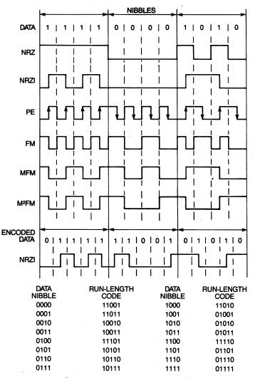
Figure 1-16 Flux-reversal codes for digital recording.
