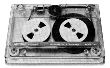
Figure 5-3 Standard <sup>1</sup>/<sub>4</sub>-inch tape cartridge.
