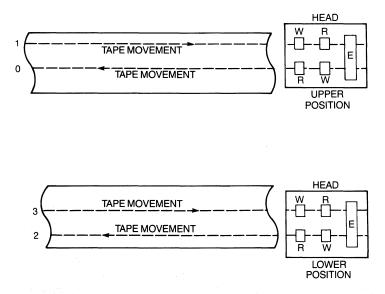
Figure 5-13 Dual-head positions for 4-track recording.
