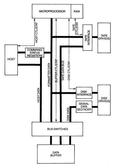
Figure 8-2 Block diagram, typical disk-tape controller.
