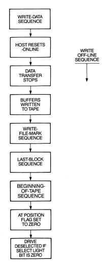
Figure 9-27 Write-Off-Line Sequence.
