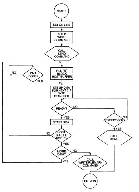
Figure 6-8 Flow diagram, write file.
