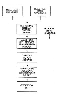
Figure 9-41 Block-In-Error Sequence.
