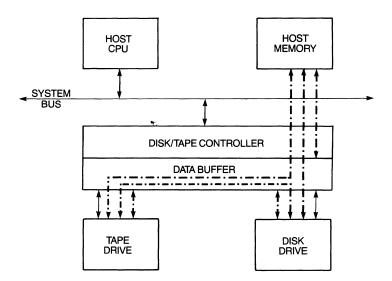
Figure 7-4 Data buffer in combined controller.
