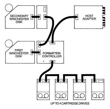
Figure 8-1 Mass-storage system with multiple disks and tape drives.
