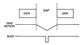
Figure 4-5 Conventional start-stop operation, <sup>1</sup>/<sub>2</sub>-inch tape.
