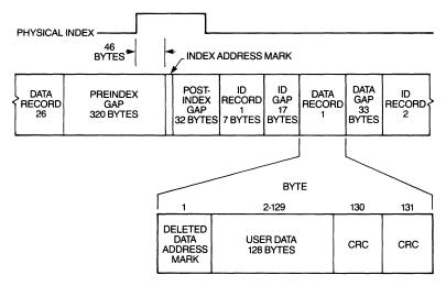
Figure 3-3 Sector format, 8-inch flexible disk.
