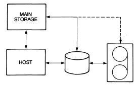
Figure 1-5 Disk storage with magnetic-tape backup.
