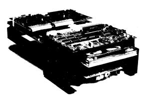
Figure 5-21 Intelligent streaming-cartridge drive.
