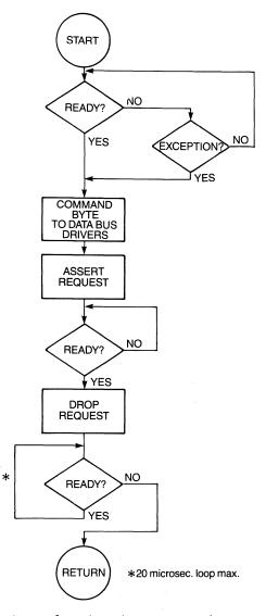
Figure 6-1 Flow diagram, send command.
