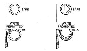
Figure 5-6 Safe and unsafe positions of write-protect plug.
