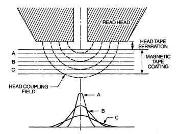
Figure 1-12 Output as a function of saturation.
