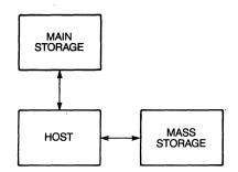
Figure 1-1 Programmed-I/O mass storage.
