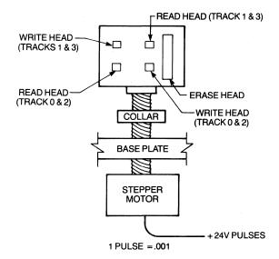
Figure 5-14 Head-positioning mechanism.
