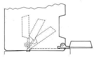
Figure 5-5 Protective door swinging open as cartridge is inserted.
