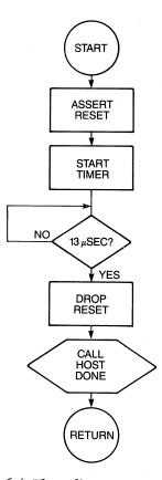
Figure 6-4 Flow diagram, reset drive.
