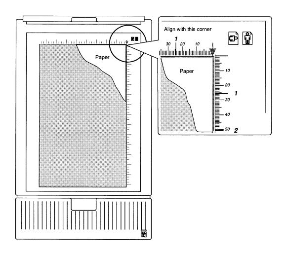
Figure 3-2 Placing the Test Chart on the Scanner
