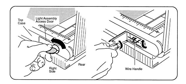
Figure 5-4 Removing the Bulb Assembly
