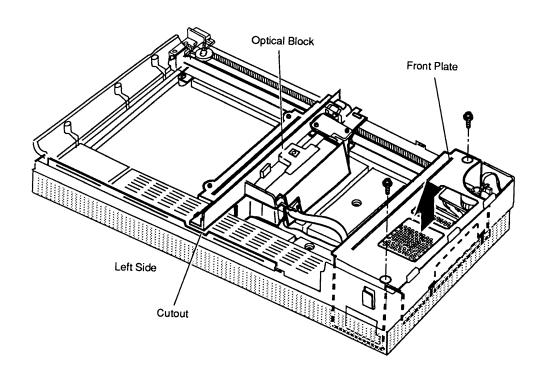
Figure 2-4 Optical Block and Front Plate
