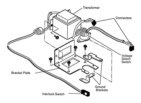
Figure 5-8 Universal Transformer Assembly
