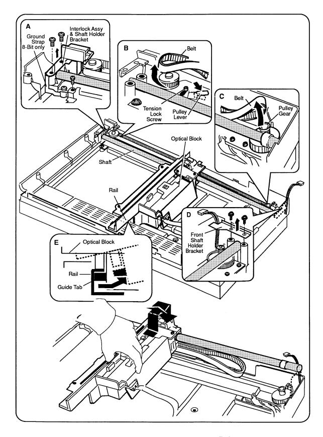
Figure 2-5 Optical Block and Drive Belt
