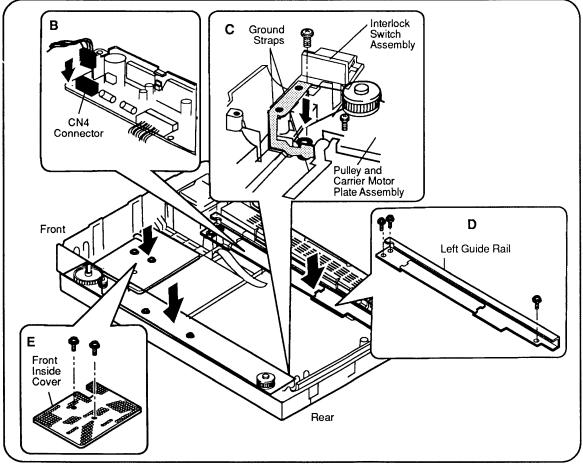
Figure 2-10 Carrier Motor
