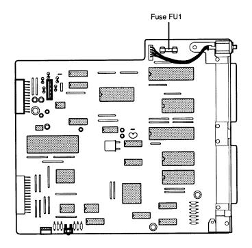
Figure 5-2 Main Logic Board Fuse on 4-Bit Scanner
