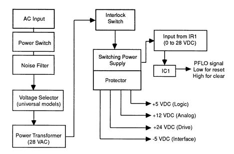
Figure 1-3 Power Circuit Block Diagram
