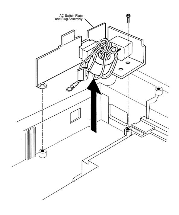
Figure 2-15 AC Switch Plate and Plug Assembly
