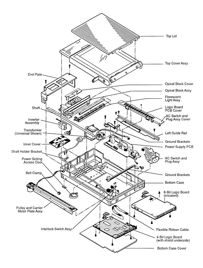
Figure 1-1 Major Assemblies and Components of the Scanner
