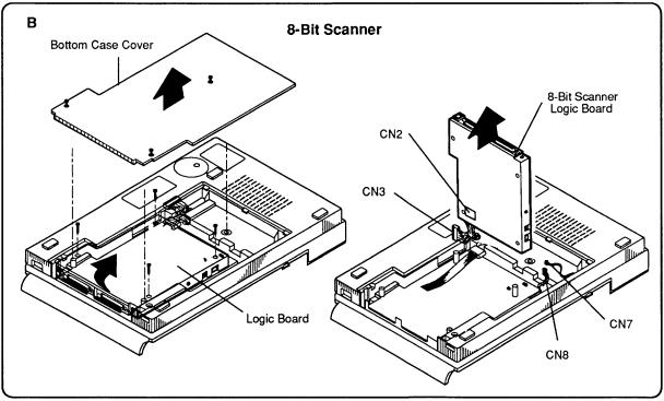
Figure 2-16 Main Logic PCB
