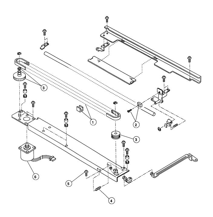
Figure 3 Carrier Assembly
