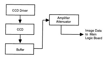
Figure 1-5 CCD PCB Block Diagram
