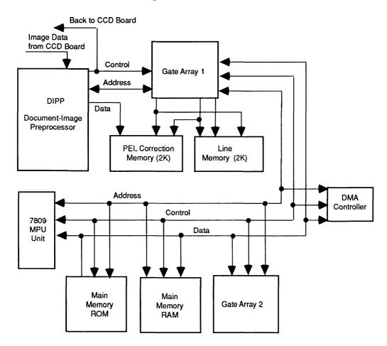
Figure 1-6 Main Logic Board Block Diagram
