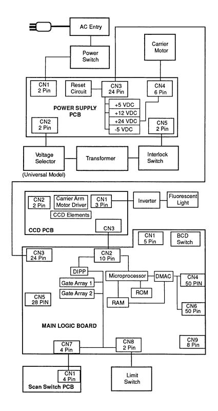
Figure 1-2 Scanner Block Diagram
