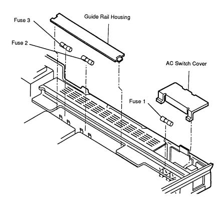
Figure 5-1 Power Supply Fuses
