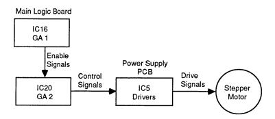
Figure 1-4 Carrier Motor Block Diagram
