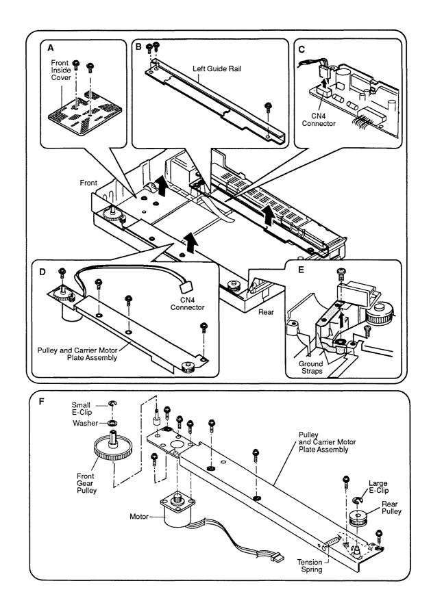
Figure 2-9 Carrier Motor
