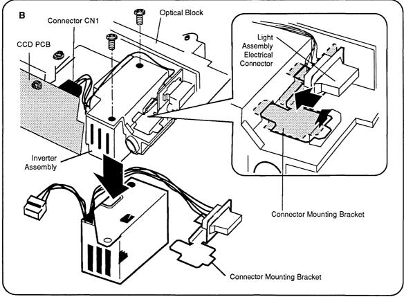
Figure 2-8 Inverter Assembly
