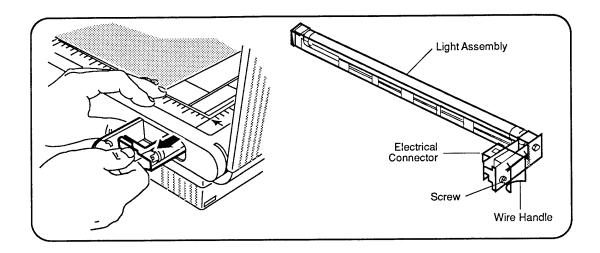
Figure 5-5 Removing the Bulb Assembly
