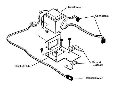
Figure 5-7 110-Volt Transformer Assembly
