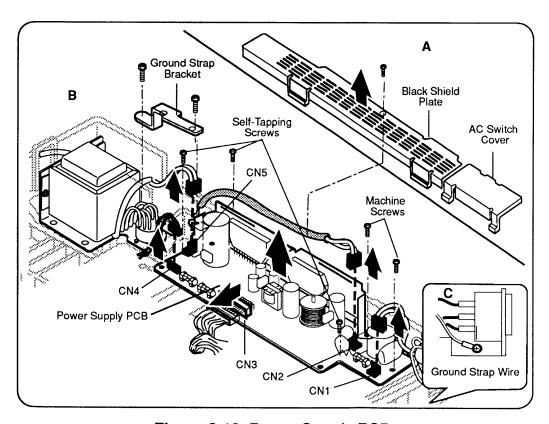
Figure 2-13 Power Supply PCB
