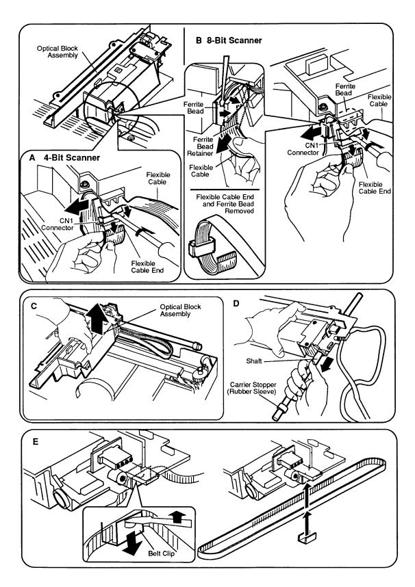
Figure 2-6 Flexible Ribbon Cable
