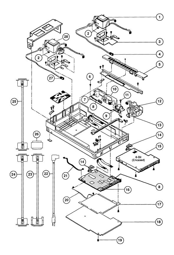
Figure 5 Cables, Power Supplies, and Logic Boards
