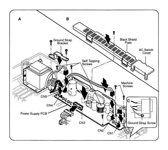
Figure 2-14 Power Supply PCB
