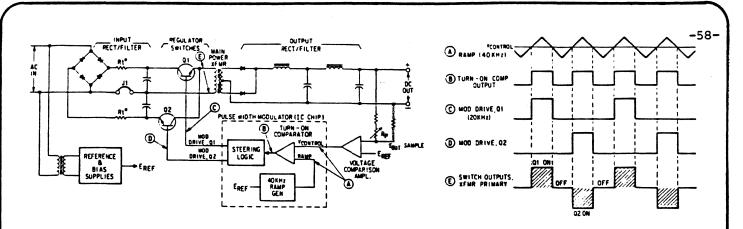
Figure 2. Switching Supply with Push-Pull Transistors and Feedback for Regulation
