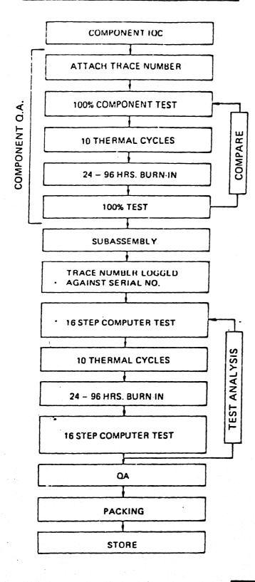
This chart details the step-by step procedures taken by ASTEC to ensure that the final product has reliability built in.
