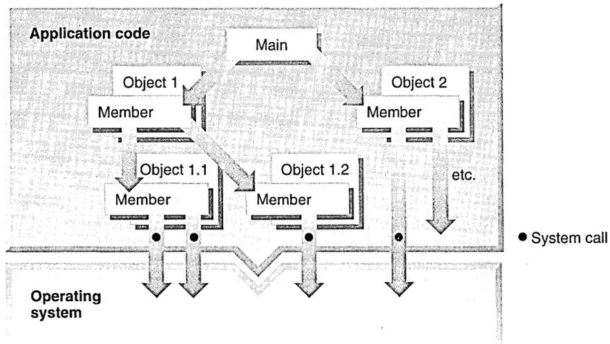
OBJECT-ORIENTED-BASED PROGRAM STRUCTURE FOR A TRADITIONAL OPERATING SYSTEM
