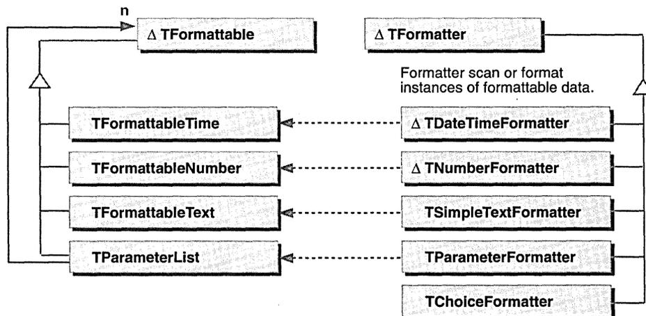
TEXT SCANNING AND FORMATTING FRAMEWORK CLASS DIAGRAM
