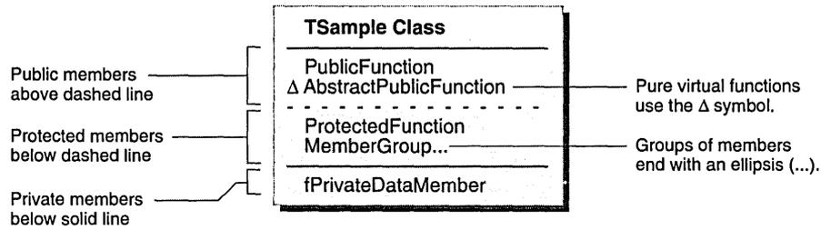
The simple class diagram below shows an example of the notation.
