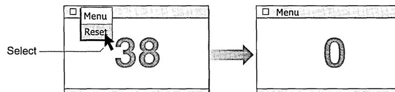
The application's menu contains a single entry, Reset, which resets the counter to 0 if selected.
