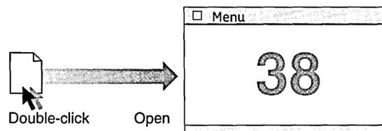
Each time the user starts the application, the number it displays is incremented from the value that it displayed the last time it was started and closed. Because the application keeps a running count, each time it is executed it provides a new value that is suitable to use, for example, as a unique serial number.
