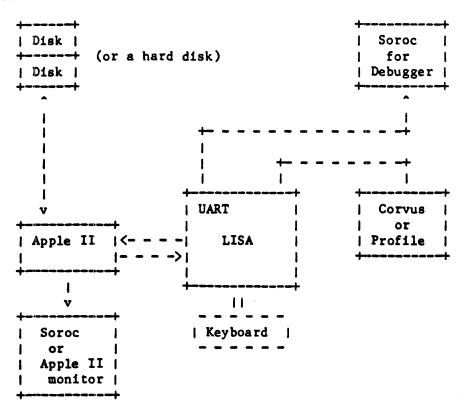
The hard disk can be connected directly to the Lisa, or it can be accessed through the Apple II. It can also be omitted.
