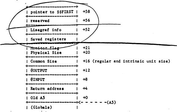
A6 is the stack frame pointer. The stack frame of a procedure is:
