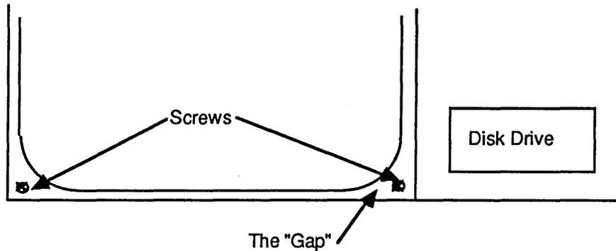
Continue pushing the inserted connector through the video compartment, through the square hole, and into the card cage compartment. Insert the four remaining connectors through the gap and into the video compartment one at a time. You might need to slightly loosen the four screws at the corners of the CRT to make the connectors fit.
