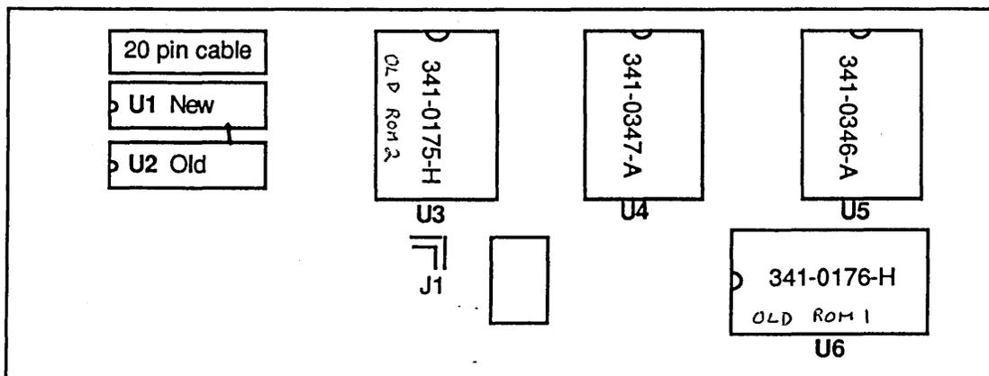
Now, the ROMSwitcher board is ready to be inserted into the XLisa CPU board. Verify that the long socket pins extending from the back of the ROMSwitcher are straight and centered. Straighten if necessary. Align the socket pins with the two empty 28-pin sockets (ROM1 & ROM2) on the XLisa CPU board. Slowly seat the socket pins into the empty sockets, being careful not to bend any of the pins. Some force may be required.
