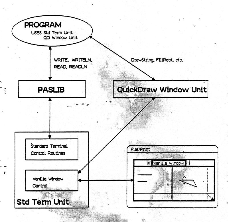
Figure 3. Data flow of WRITELNS, READLNS and QuickDraw output to a vanilla window from a program that uses the Vanilla Window/Standard Terminal Unit and the QuickDraw Window Unit.
