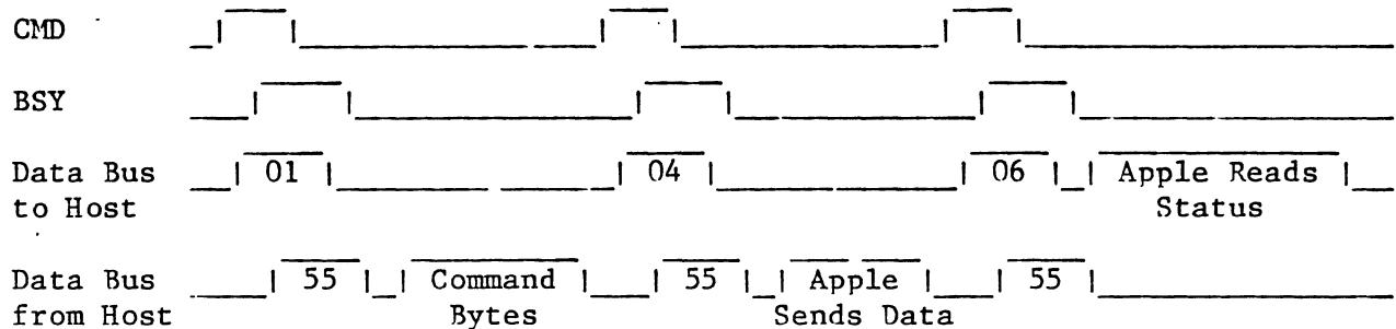
Important: The host must raise CMD following the last operation requested, since changes in Profile's spâre and bad block tables do not get rewritten onto the disk until this occurs.
