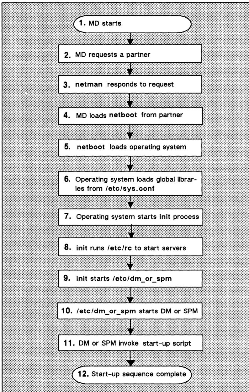
Figure 3-3. The Start-Up Sequence for a Diskless Node
