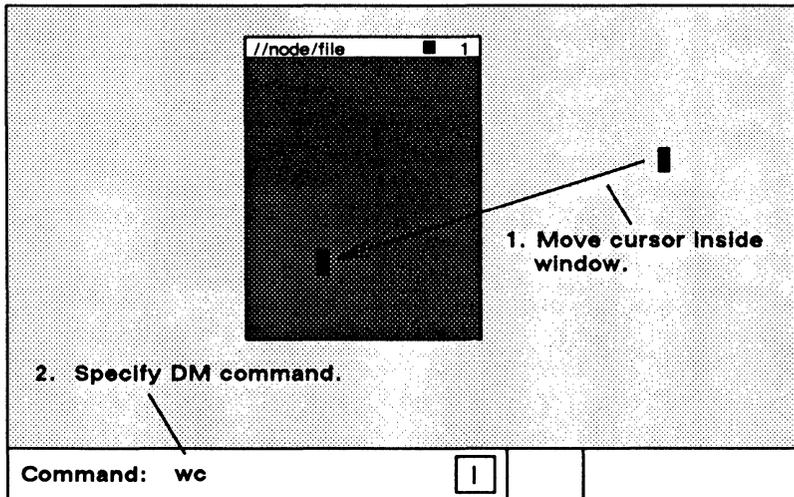
*Figure 4-1. Invoking a DM Command Interactively*
