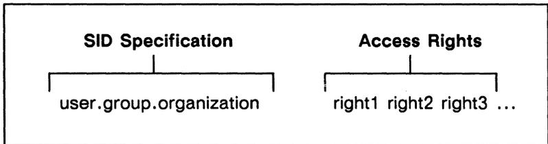
*Figure 14-1. Structure of an ACL Entry*
