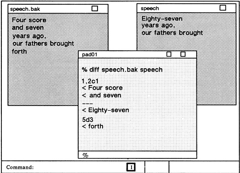
*Figure 11-3. Comparing Two ASCII Files*
