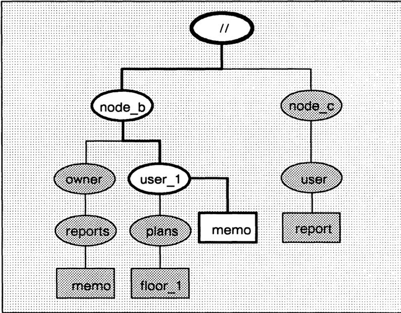
Figure 1-3. A Sample Path Through the Naming Tree
