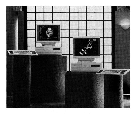
The 19" monitors are used for higher resolution (1280x1024) monochrome and higher resolution color graphic subsystems as well as the "F" option—a 2-D accelerator used for increased graphics drawing capabilities. One 19" color monitor operates at 70Hz refresh rate and is used in conjunction with the 8-plane Desktop Visualization System graphics option.
