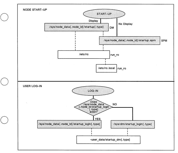
Note: Solid lines (---) indicate automatic operations. Dashed lines (---) indicate paths where the preceding file must specify the following file (for example, /etc/rc must specify /etc/rc.local). Program names to the right of a file (e.g., run\_rc or DM) indicate the program that executes the commands in the file.
