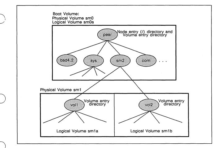
Figure 3-2. A node with Multiple Physical and Logical Volumes
