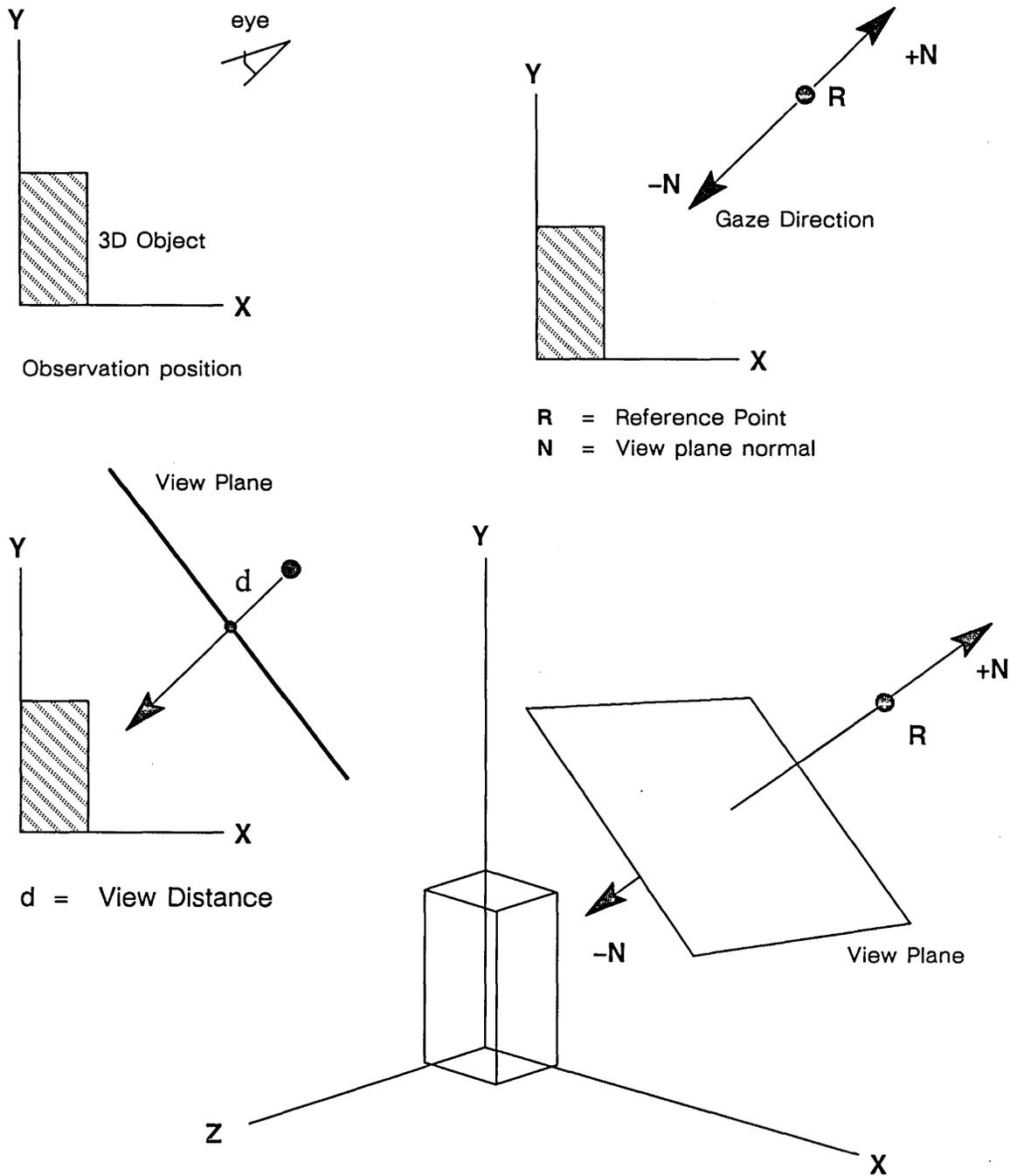
Figure 7-3. Specifying the View Plane in a Right-Handed System
