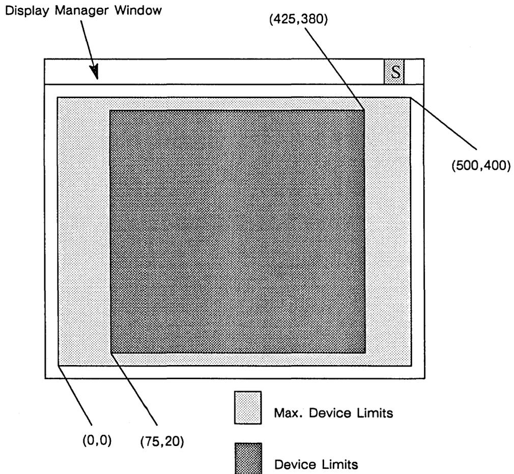
Figure 8-2. Maximum Device Limits and Device Limits
