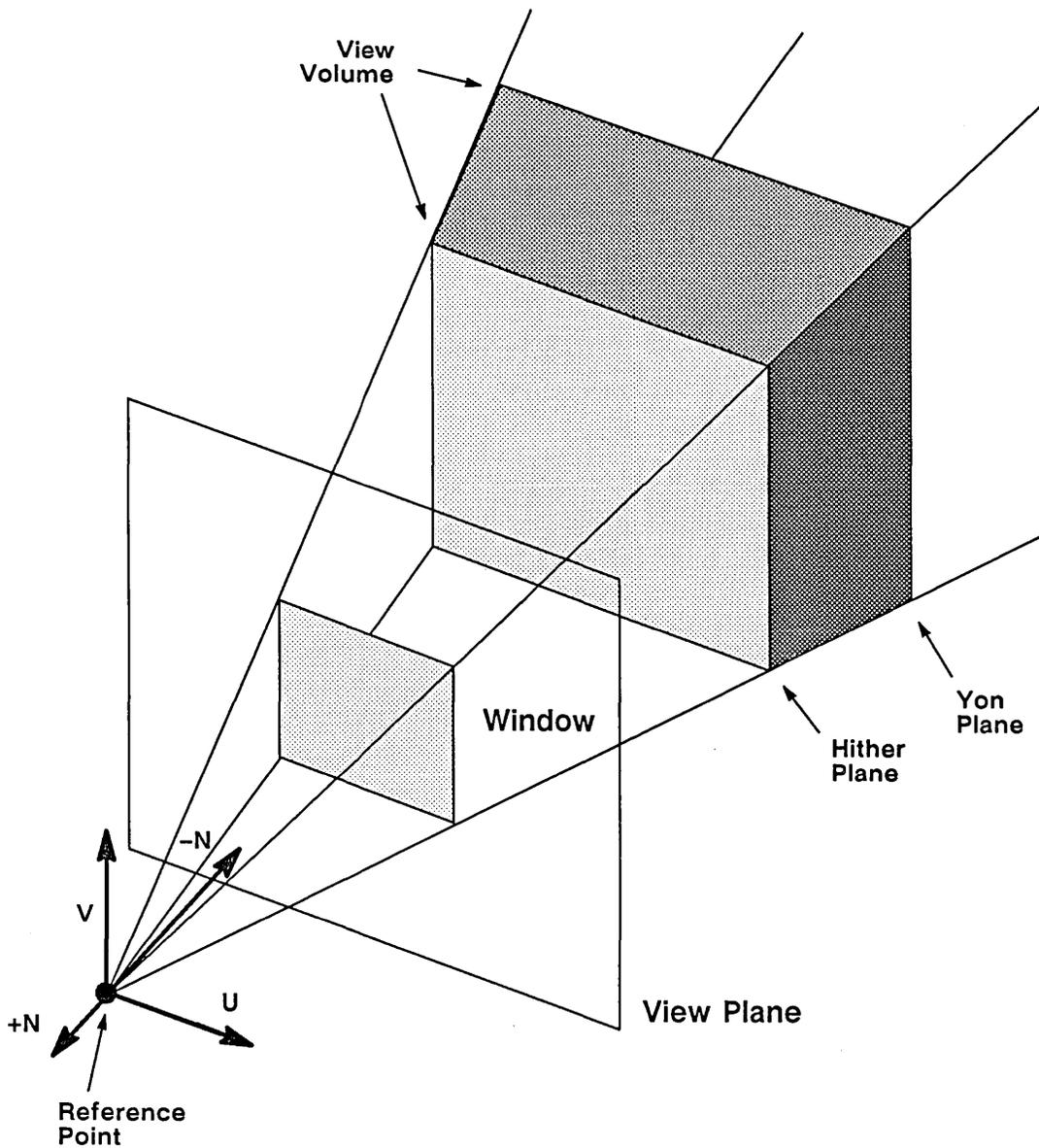
Figure 7-12. Right-handed Perspective Projection View Volume
