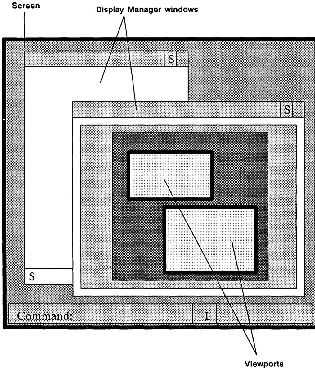
Figure 1-3. Direct Mode Displays within a DM Window
