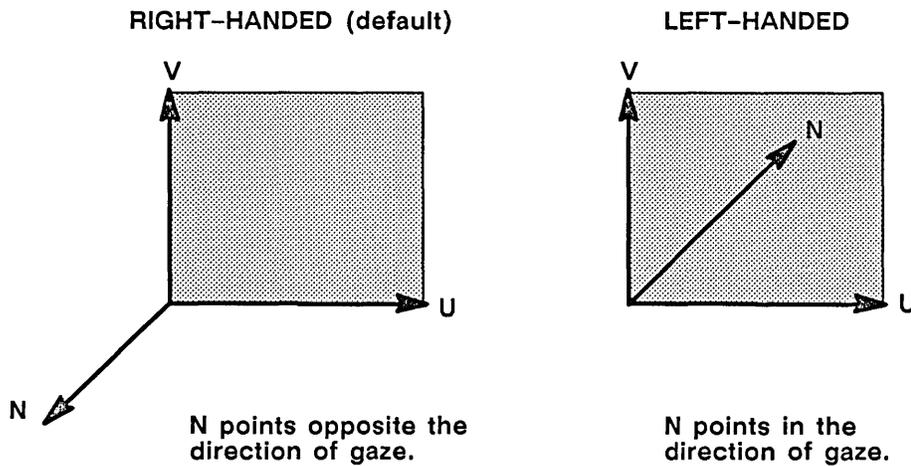
Figure 7-4. Right- and Left-handed Viewing Coordinate Systems
