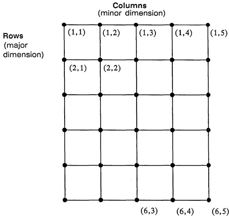
Figure 3-1. A Mesh with 5x4 Quadrilaterals Requires 30 Points
