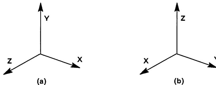
Figure 1-6. Examples of Right-handed World Coordinate Systems
