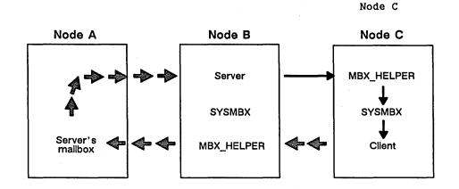
Figure 5-13. How MBX\_HELPER Assists Interprocess Communication
