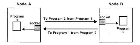
Figure 6-1. Using Sockets to Receive Datagrams
