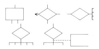
**4.10.2** *Multiple Logic Paths.* Each exit from a symbol shall be identified to show the logic path which it represents. The logic paths may be represented by a table that indicates their associated conditions and the inconnector references.
