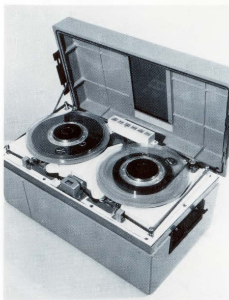
The ATM-13, one of the Ampex high environment series, is a lightweight, closed-loop digital tape drive employing a variation of the Ampex single capstan tape drive and patented electronic servo control. Two vacuum chambers (underneath the two tape reels) provide uniform tension to hold the tape in constant contact with the capstan drive, ensuring positive head-to-tape contact. The ATM-13 is the only unit of its type capable of recording blocks of digital data suitable for conventional computer format.
