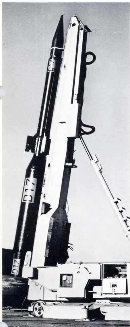
Solid propellant Dragon sounding rocket on its launching pad. This is one of an extensive range of space probes launched by France.
