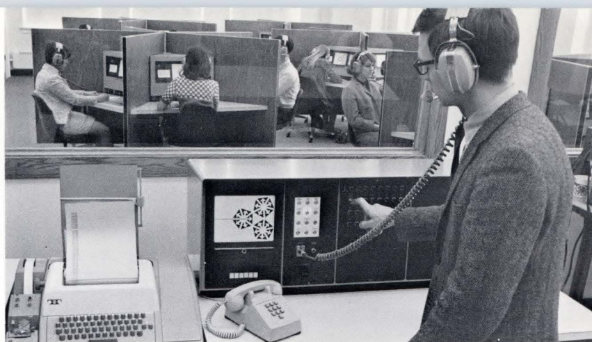
Technical supervisor at master control console, used when attended operation instead of the fully automatic control is desired. All student controls are duplicated here so that the supervisor can take over or share control. Teletype at left logs out program numbers and is used during diagnostic programs for readout.
