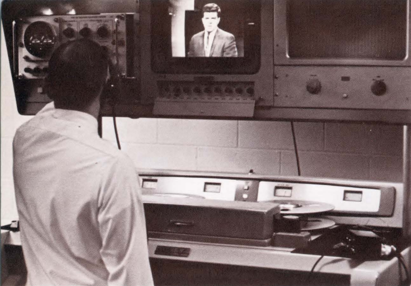
Technician adjusts monitoring oscilloscope on one of the six VR-1000C recorders used by the Delaware ETV Network.
