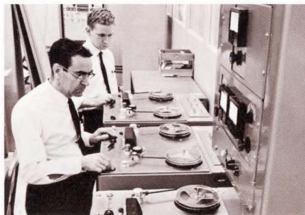
Ampex Model 3200 duplicator makes copies of audio tapes for New York schools.
