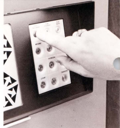
The student selects mode of operation (program number, play, stop, recue at beginning) by push buttons. System is immune to pranksters because the student doesn't operate the equipment directly. All commands are routed by a computer which controls the entire system.
