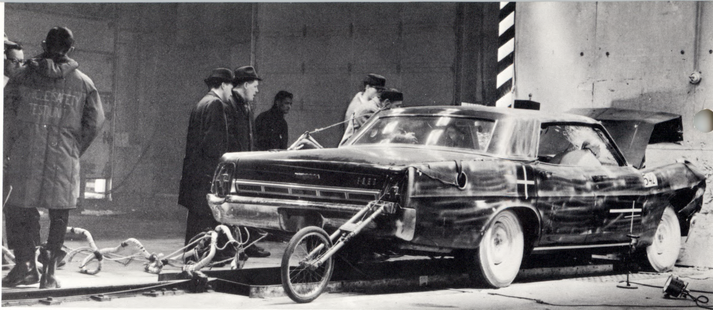
Ford engineers examine a 1967 Ford after it has impacted a 200-ton concrete barrier at 30 mph.
