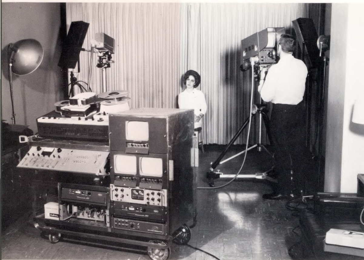
Recording and control equipment in the Psychiatric Department is all contained on two mobile carts, each with an Ampex VR-660 recorder, three monitors, a control board, and associated devices. These carts can be easily moved to a patient's room or to other locations as needed.
