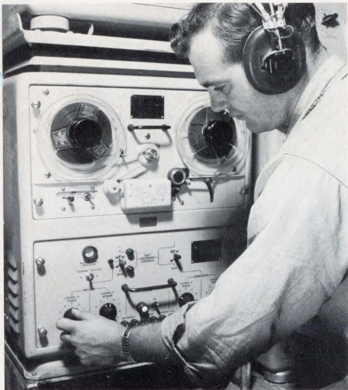
An Ampex UNQ-7 dual-track recorder in operation aboard a U.S. Navy submarine. This rugged machine is used to record and playback audio-frequency data in a variety of special Navy installations.
