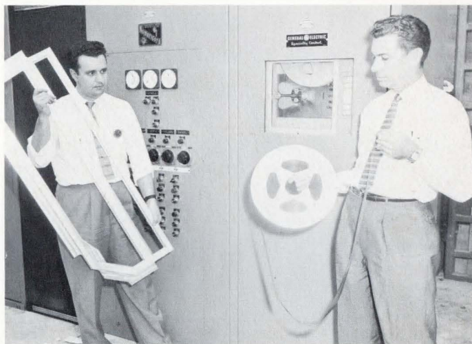
At CONVAIR, Ft. Worth, an engineer holds the roll of magnetic tape used to control the machinery which turned out the B-58 wing slug held by the man at left.
