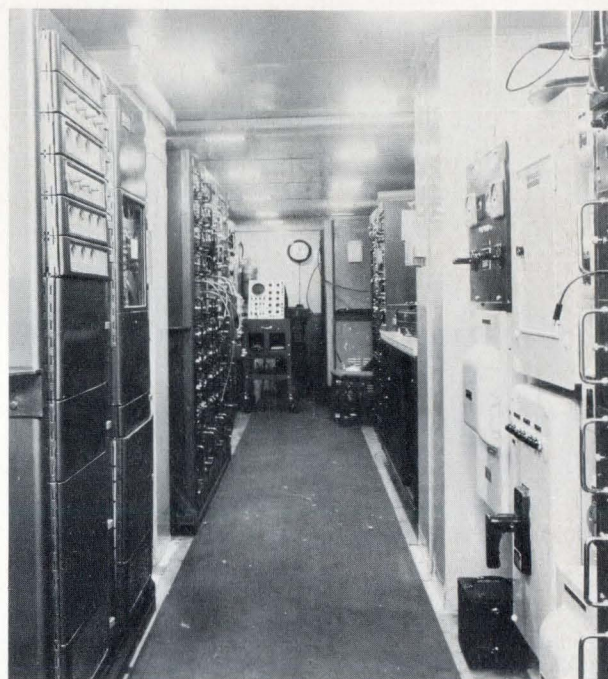
A trailer-van installation used in Florida by GENERAL ELECTRIC Missile & Ordnance System Department. FR-100 recorders collect data from nose-cone instruments in missile firings.
