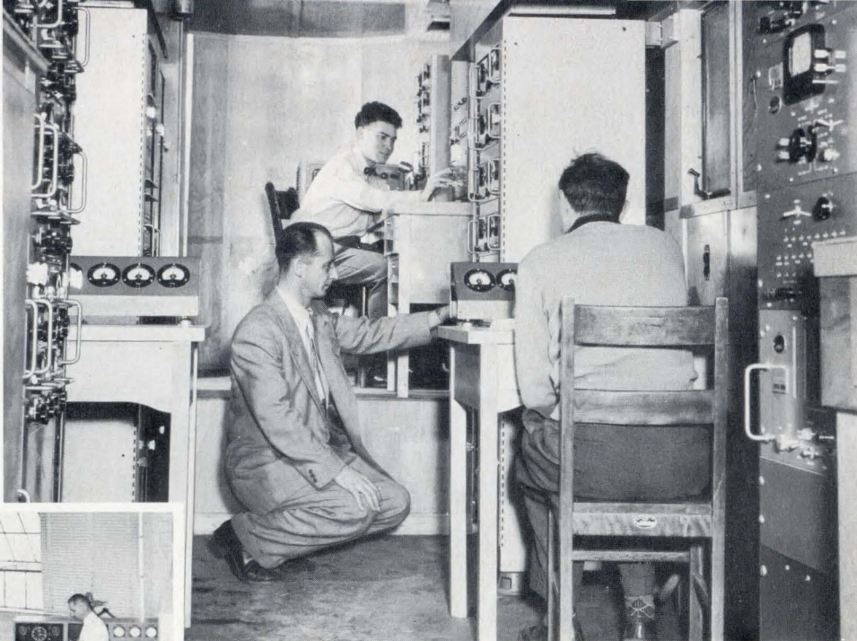
A portion of instrumentation-van equipment used in conjunction with Ampex recorders at AVRO CANADA for receiving and processing telemetered flight test data.
