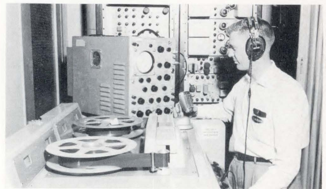
An Ampex Videotape recorder, in use at WHITE SANDS PROVING GROUND Electronics Warfare Division, is employed for such purposes as recording radar emissions from a missile in flight.
