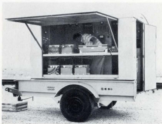
A trailer-mounted instrumentation laboratory designed by a nuclear weapons development laboratory for use on a desert proving ground, employing a Model 800 14-track recorder.
