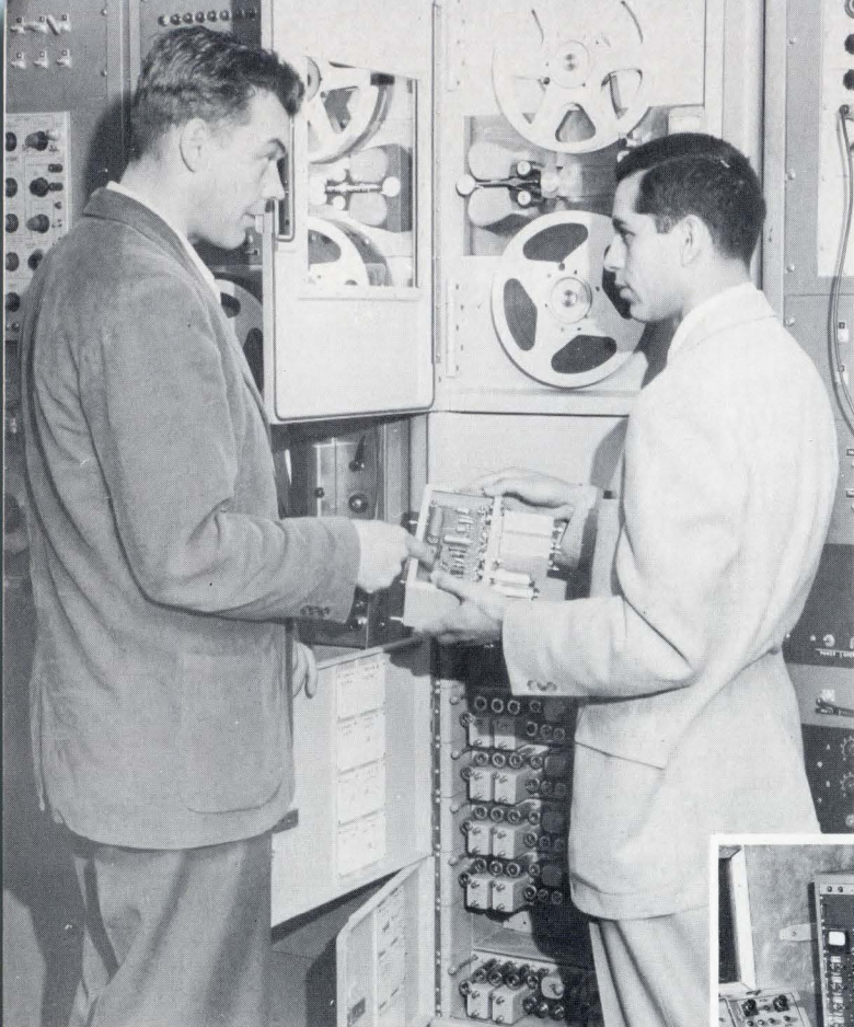
An engineer at WHITE SANDS PROVING GROUND demonstrates the modular plug-in units of an FR-100 instrumentation recorder used in an extensive data-reduction facility.
