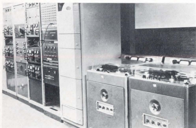
For the REPUBLIC AVIATION data-processing facility at Farmingdale, Connecticut, an Ampex 14-inch-reel transport with 1-inch tape is teamed with a \frac{1}{4} -inch tape transport, both servo speed controlled and equipped for direct, PDM and FM recording. The tape transport at left may be adapted for use with a continuous loop of tape, for maximum utility in complex-wave analysis.
