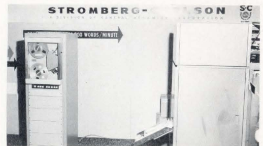
For translating computer data into printed copy at rates as high as 100,000 words per minute, the STROMBERG-CARLSON S-C 5000 Printer uses an FR-400 digital tape handler.
