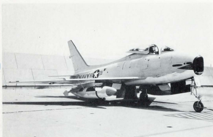
The wing tank on this NORTH AMERICAN AIRCRAFT FJ-4 holds a Model 800 recorder, and permits rapid transfer of the complete recording installation from one plane to another.
