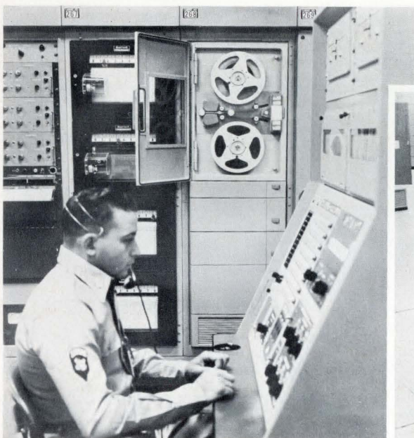
Simulation system at the U.S. Army's Talos unit, WHITE SANDS PROVING GROUND, New Mexico, which uses Ampex instrumentation recorders to simulate enemy attacks and to train operating personnel.
