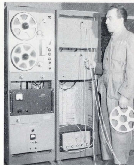
An installation in Milan, Italy, at Laboratory Gomma facilities of SOCIETA PIRELLI. The instrumentation recorder here serves in intensive tire-research programs.
