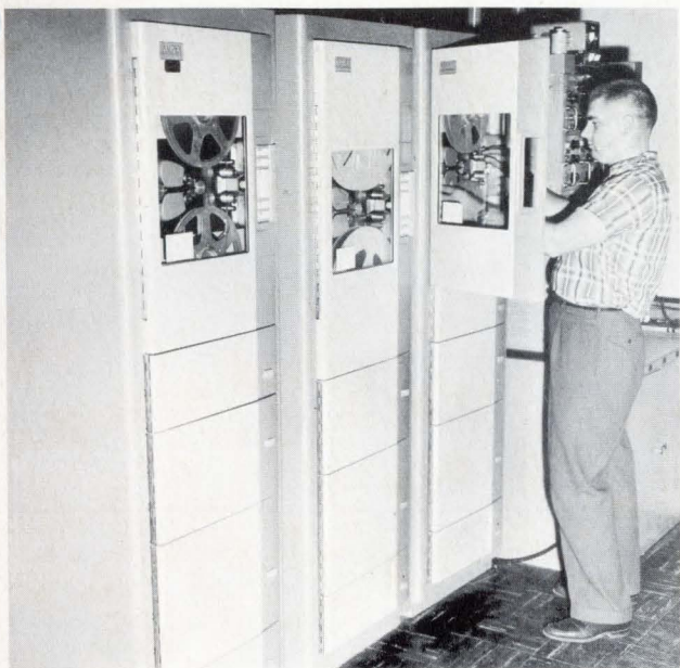
A bank of FR-100 recorders at the U.S. NAVAL MINE DEFENSE LABORATORY at Panama City, Florida. These instruments reproduce tapes recorded by on-the-spot data-acquisition recorders.
