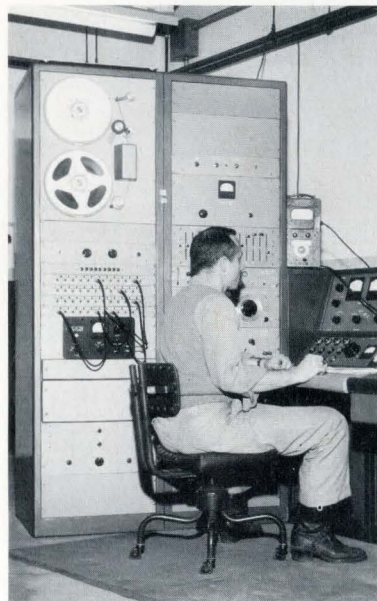
FR-100 recorders in a digital data processing system to be used with flight simulation tests at HOLLOMAN AFB, New Mexico.
