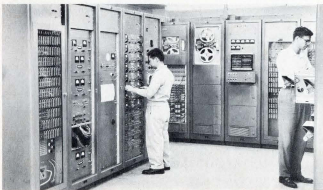
DOUGLAS AIRCRAFT COMPANY's test facilities near Sacramento, California, where FR-100 recorders are used to process data acquired by other Ampex recorders located at missile static-test firing sites.
