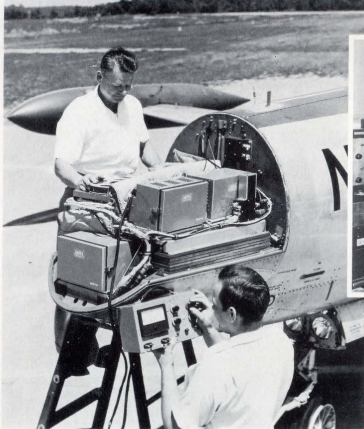
Ground station playback system, employing Model 300 and FR-100 equipment, in use at the NACA Cleveland facility.
